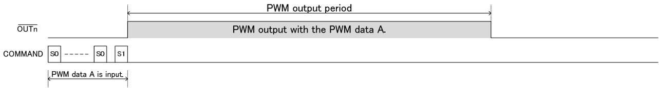
When doing PWM output once again, it's necessary to input S1 command.
