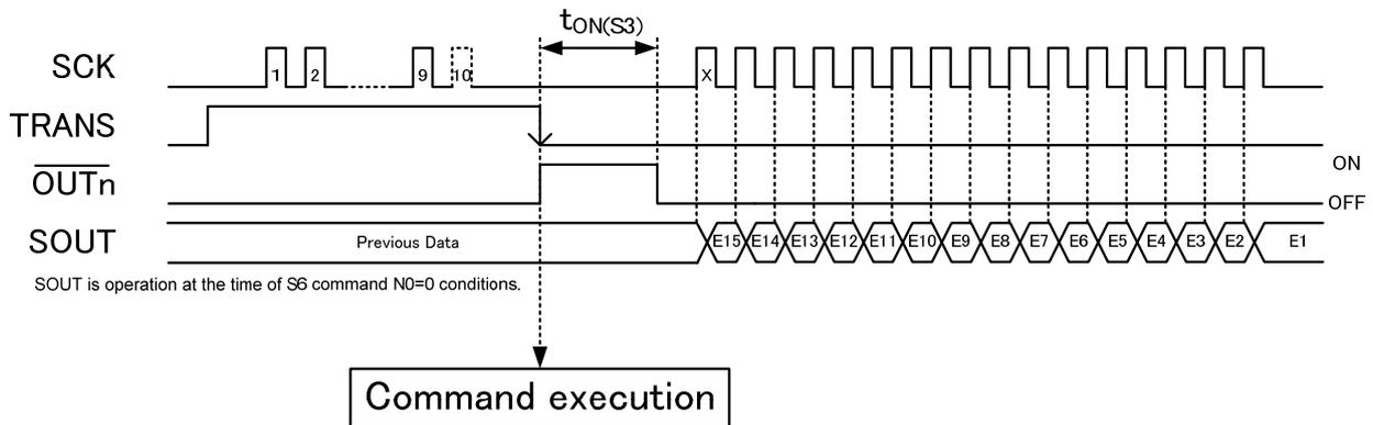
The first SCK (signal X) after this command is used for transmission of the output open/short detection result data. The input from SIN is not received. Note1
