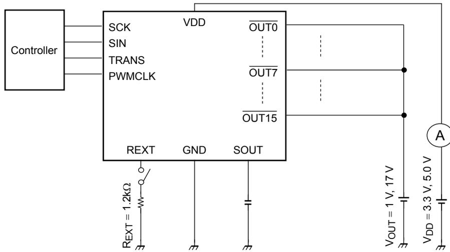
Test circuit 5 : Constant current error / Output OFF leak current
