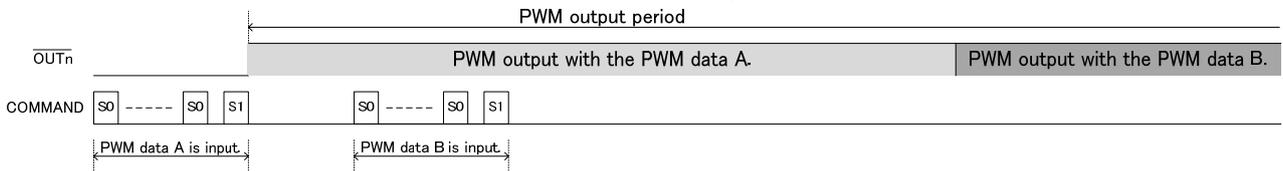
If S1 command is inputted two or more times during a PWM output by PWM output synchronous mode, after the present PWM output has ended, a PWM output will be started by the PWM data inputted at the end.
