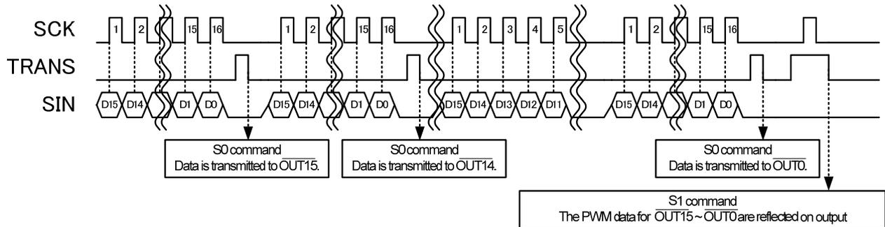
**3-2) Speed input mode (S0 command 15 times + S1 command once)**
