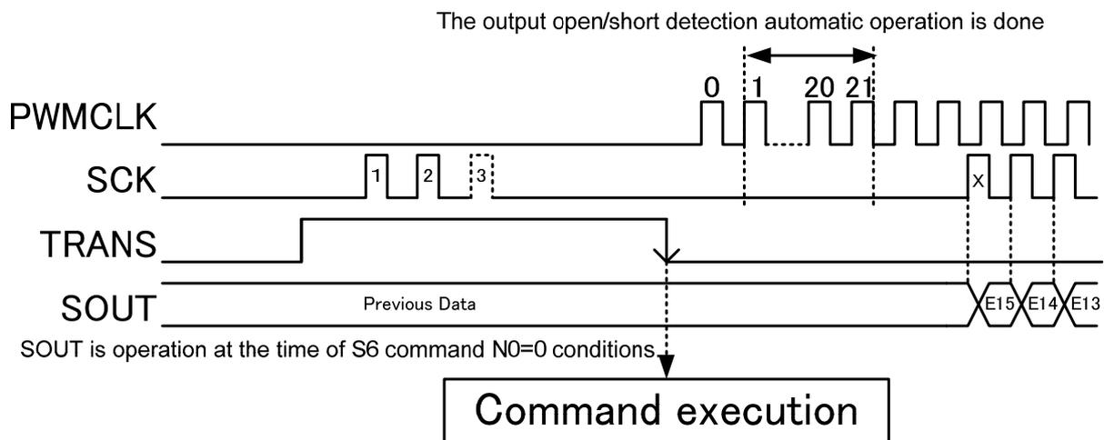
The first SCK (signal X) after S1 command is used for transmission of the output open/short detection result data. The input from SIN is not received. Note1
