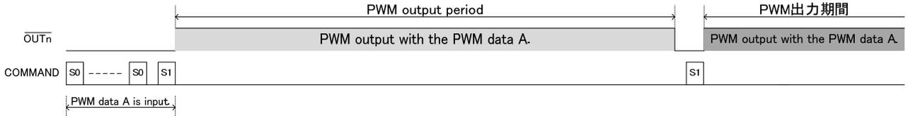
When S1 command is inputted during a PWM output by PWM output asynchronous mode, the present PWM output is canceled and a PWM output is immediately started by new PWM data.
