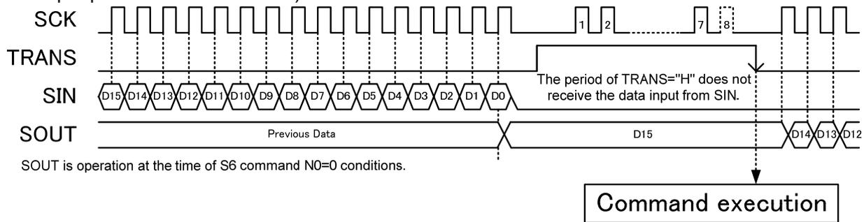
Note1: PWM output synchronization PWM resolution is set by the S6 command.
