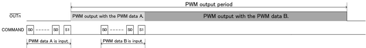
When S1 command is inputted during a PWM output by PWM output synchronous mode, after the present PWM output has ended, a PWM output is started by new PWM data.
