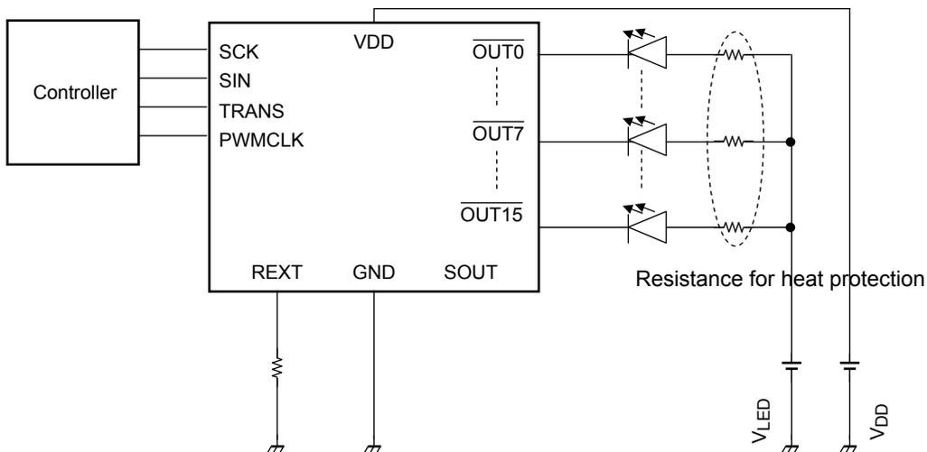
**Setting method of resistance for heat protection**
