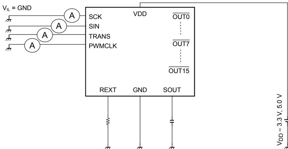
Test circuit 4 : Power supply current
