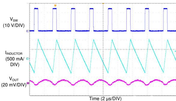
$V_{IN} = 24\text{ V}$  |  $V_{OUT} = 5\text{ V}$  |  $f_{SW} = 400\text{ kHz}$
