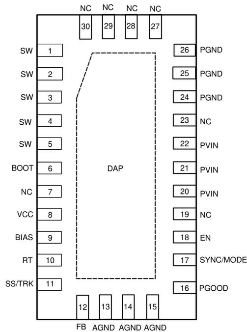
**Figure 5-1. RNP Package 30-Pin WQFN Top View**
