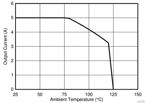
**Figure 8-3. LM76005-Q1 Safe Operating Area (5 V<sub>OUT</sub>, 400 kHz, R<sub>θJA</sub>=18.8 °C/W)**
