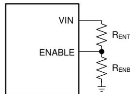
Figure 7-3.  $V_{IN}$  UVLO
