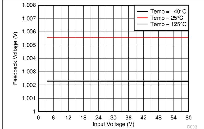
**Figure 6-3. Feedback Voltage**
