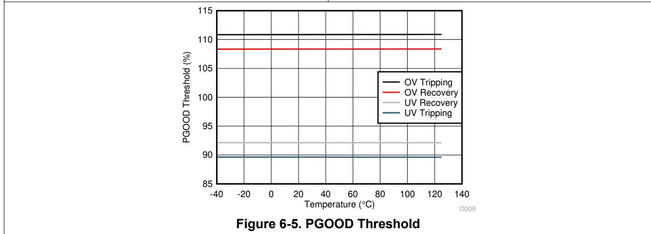
**Figure 6-5. PGOOD Threshold**
