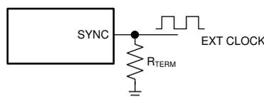
**Figure 7-7. Frequency Synchronization**
