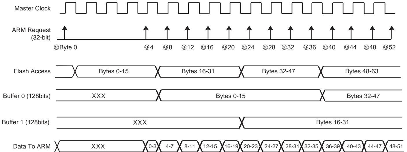
Note: When FWS is included between 1 and 3, in case of sequential reads, the first access takes (FWS+1) cycles, the other ones only 1 cycle.
