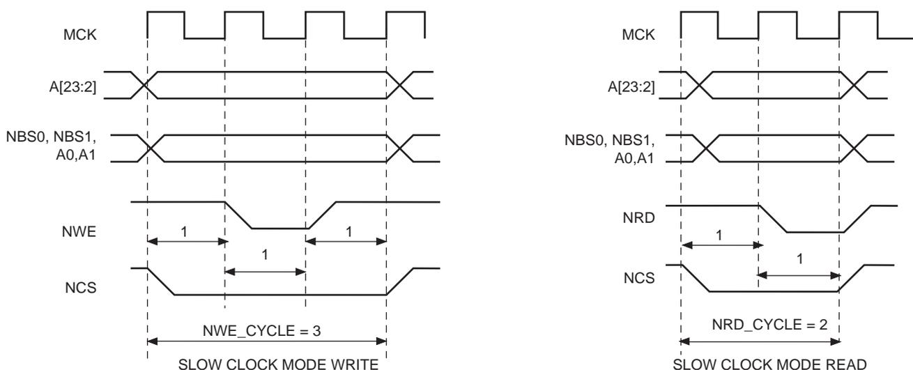
Table 24-8. Read and Write Timing Parameters in Slow Clock Mode
