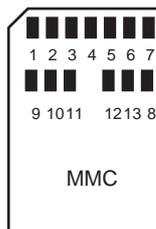
The High Speed MultiMedia Card communication is based on a 13-pin serial bus interface. It has three communication lines and four supply lines.
