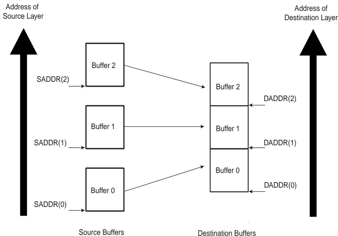
The DMAC transfer flow is shown in [Figure 39-9 on page 1018](#).
