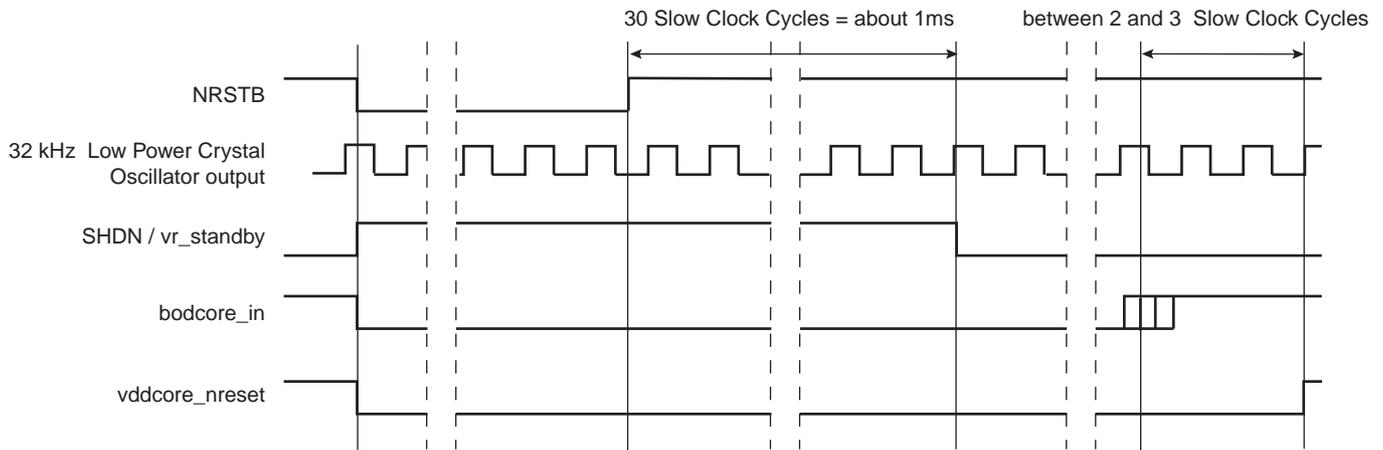
Note: periph\_nreset, ice\_reset and proc\_nreset are not shown, but are asserted low thanks to the vddcore\_nreset signal controlling the Reset controller.
