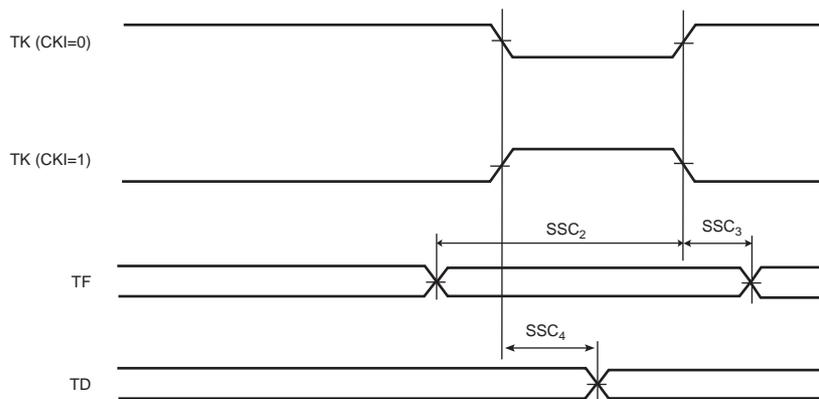
**Figure 42-24. SSC Transmitter, TK and TF as Input**
