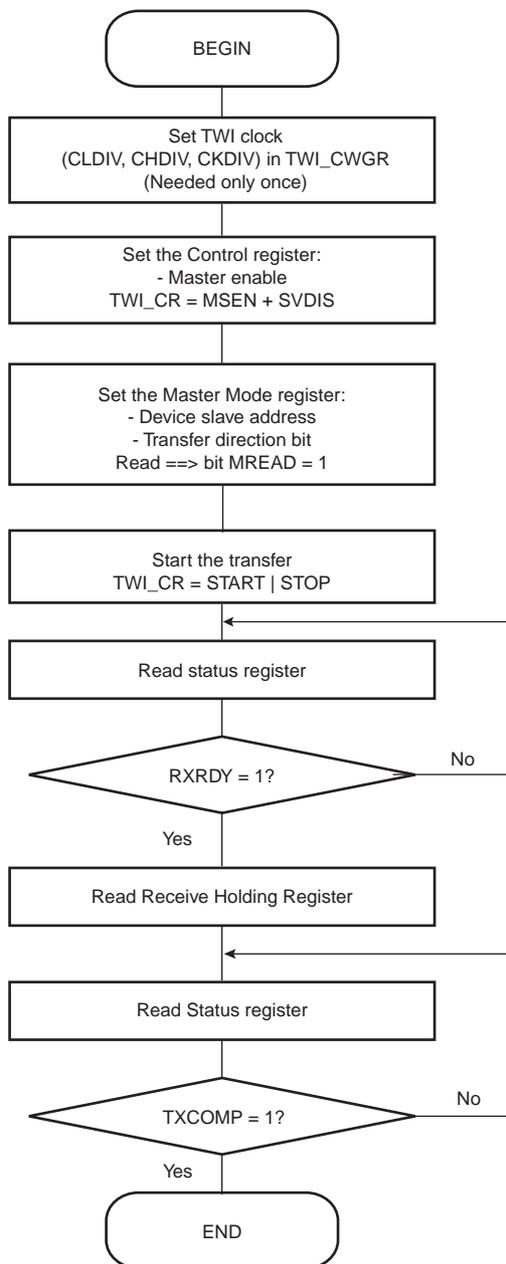
Figure 32-19. TWI Read Operation with Single Data Byte and Internal Address
