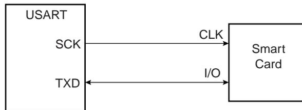
When operating in ISO7816, either in T = 0 or T = 1 modes, the character format is fixed. The configuration is 8 data bits, even parity and 1 or 2 stop bits, regardless of the values programmed in the CHRL, MODE9, PAR and CHMODE fields. MSBF can be used to transmit LSB or MSB first. Parity Bit (PAR) can be used to transmit in normal or inverse mode. Refer to “USART Mode Register” on page 730 and “PAR: Parity Type” on page 731.
