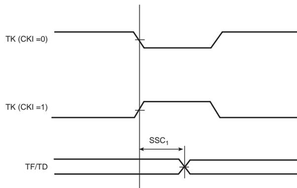
**Figure 42-23. SSC Transmitter, TK as Output and TF as Input**
