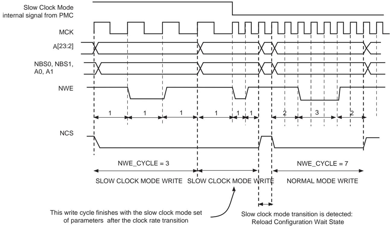
**Figure 24-30. Recommended Procedure to Switch from Slow Clock Mode to Normal Mode or from Normal Mode to Slow Clock Mode**
