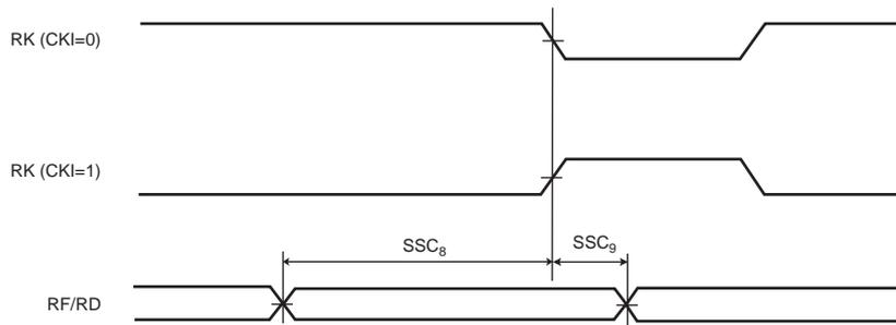
**Figure 42-26. SSC Receiver, RK as Input and RF as Output**
