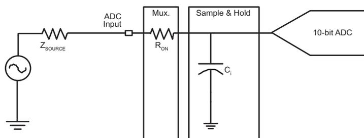
The user can drive ADC input with impedance up to:
