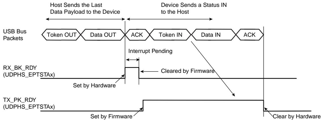
Note: Before proceeding to the status stage, the software should determine that there is no risk of extra data from the host (data stage). If not certain (non-predictable data stage length), then the software should wait for a NAK-IN interrupt before proceeding to the status stage. This precaution should be taken to avoid collision in the FIFO.
