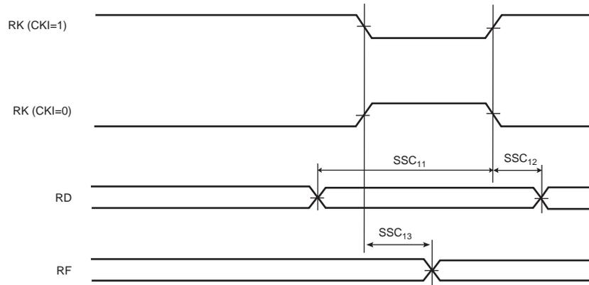
**Figure 42-28. SSC Receiver, RK as Output and RF as Input**
