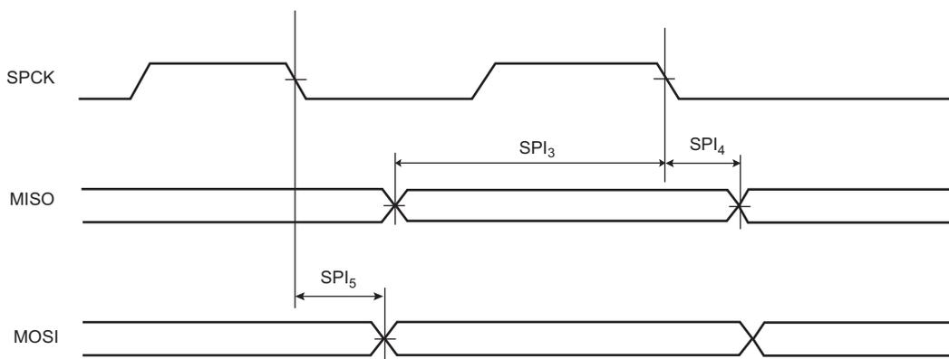
**Figure 42-19. SPI Slave Mode with (CPOL = 0 and NCPHA = 1) or (CPOL = 1 and NCPHA = 0)**
