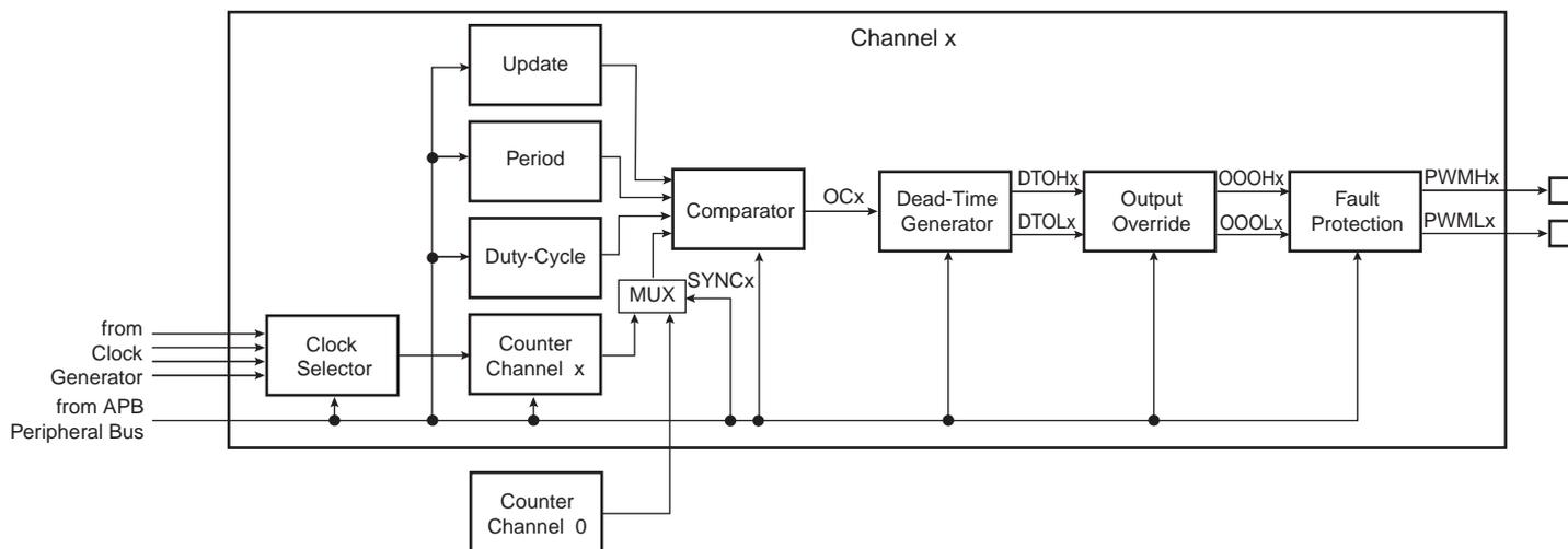
Each of the 4 channels is composed of six blocks:
