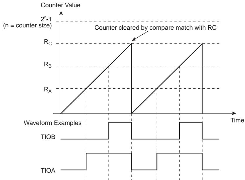
**Figure 35-10. WAVSEL = 10 with Trigger**
