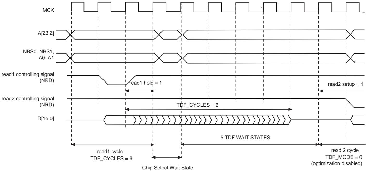
**Figure 24-21. TDF Mode = 0: TDF wait states between a read and a write access on different chip selects**
