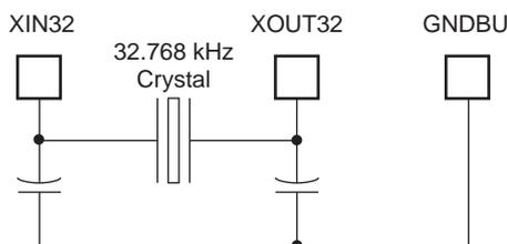
The user can set the Slow Clock Crystal Oscillator in bypass mode instead of connecting a crystal. In this case, the user has to provide the external clock signal on XIN32. The input characteristics of the XIN pin under these conditions are given in [Section 42. "Electrical Characteristics"](#).
