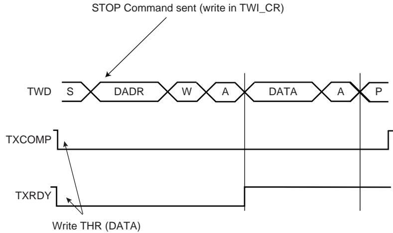
**Figure 32-7. Master Write with Multiple Data Bytes**
