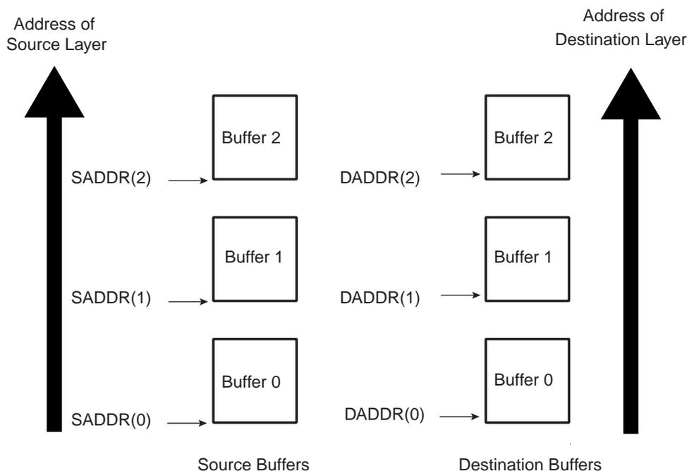
If the user needs to execute a DMAC transfer where the source and destination address are contiguous but the amount of data to be transferred is greater than the maximum buffer size DMAC\_CTRLAx.BTSIZE, then this can be achieved using the type of multi-buffer transfer as shown in [Figure 39-6 on page 1014](#).
