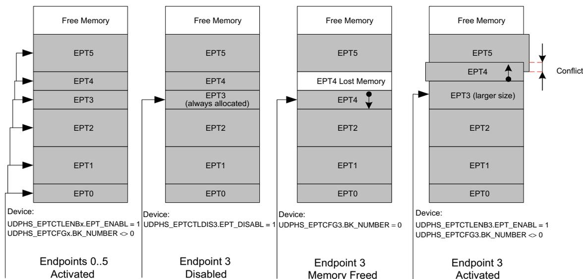
1. The endpoints 0 to 5 are enabled, configured and allocated in ascending order. Each endpoint then owns a memory area in the DPRAM.
