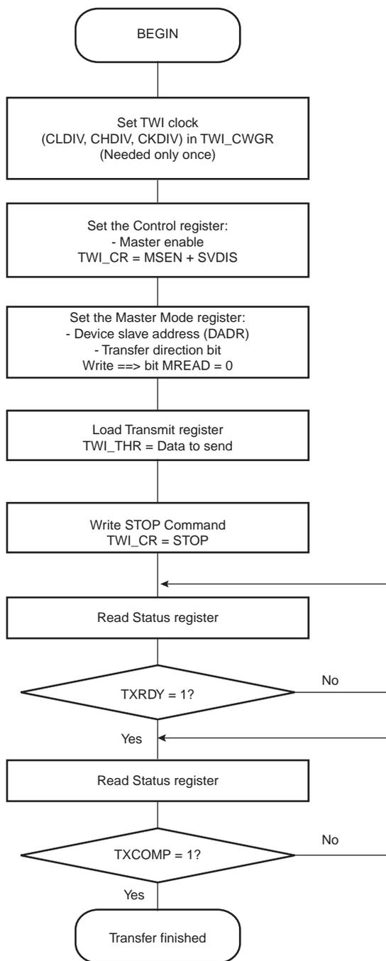
Figure 32-16. TWI Write Operation with Single Data Byte and Internal Address
