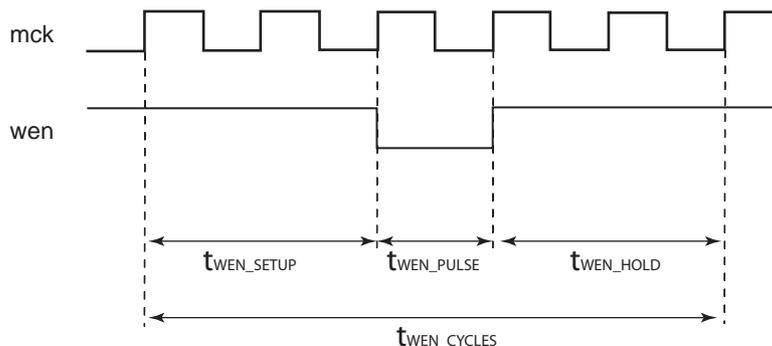
**Figure 24-33. Write Enable Timing for NAND Flash Device Data Input Mode.**
