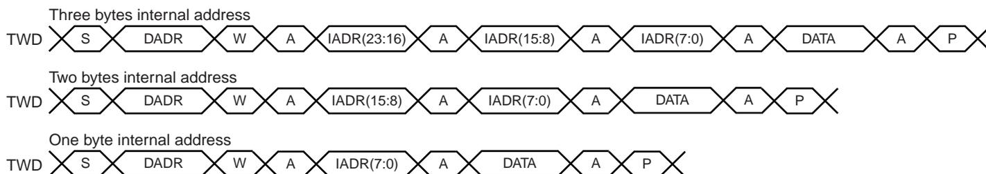
**Figure 32-12. Master Read with One, Two or Three Bytes Internal Address and One Data Byte**
