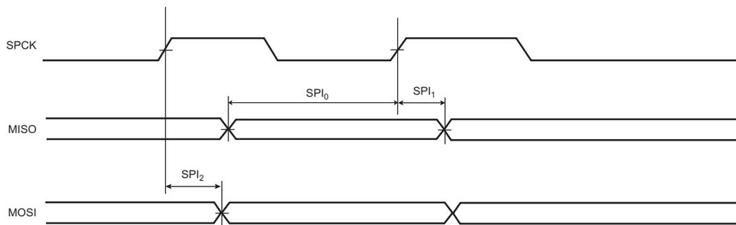
**Figure 42-18. SPI Master Mode with (CPOL = 0 and NCPHA = 1) or (CPOL = 1 and NCPHA = 0)**
