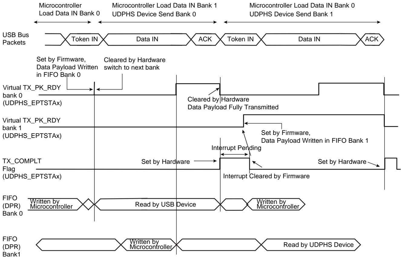
**Figure 38-10. Data IN Followed By Status OUT Transfer at the End of a Control Transfer**
