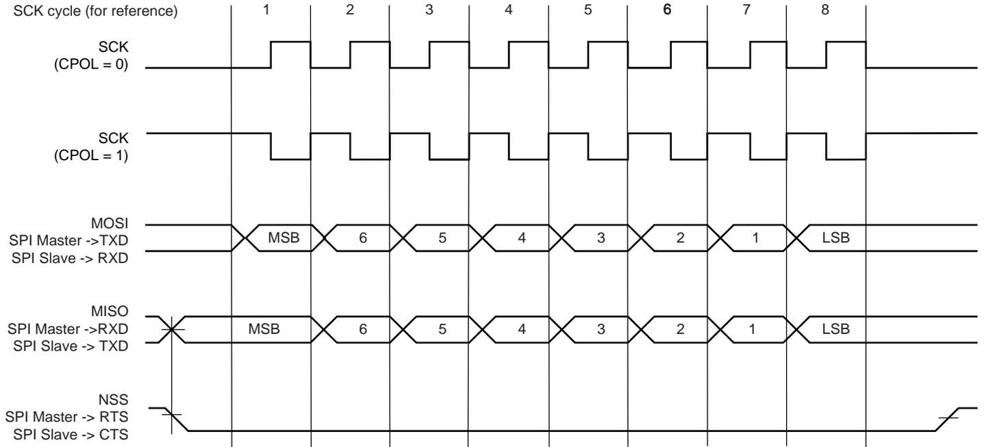
**Figure 34-39. SPI Transfer Format (CPHA=0, 8 bits per transfer)**
