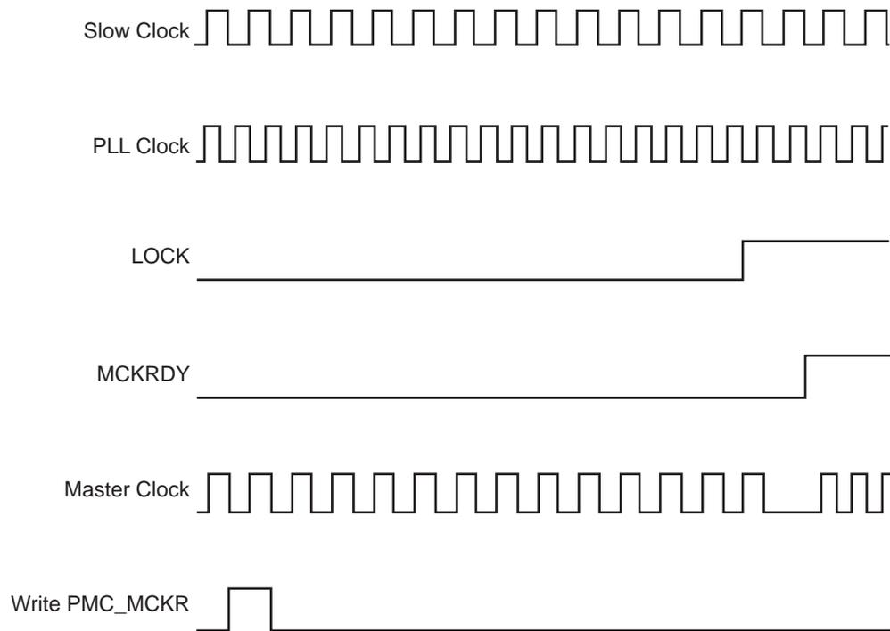
**Figure 27-5. Switch Master Clock from Main Clock to Slow Clock**
