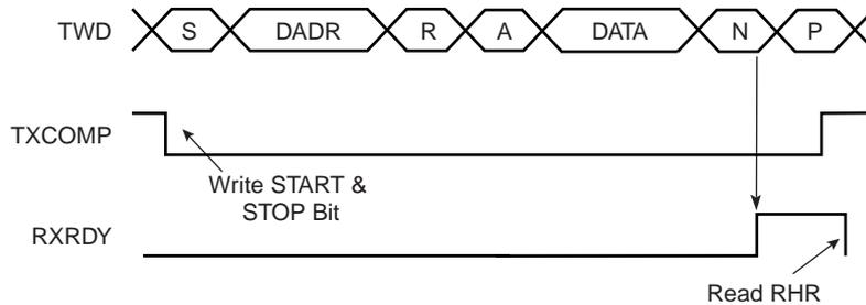
**Figure 32-10. Master Read with Multiple Data Bytes**
