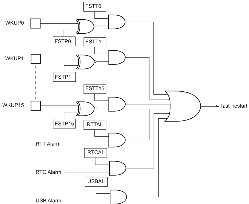
Each wake-up input pin and alarm can be enabled to generate a Fast Startup event by setting the corresponding bit in the Fast Startup Mode Register (PMC\_FSMR).
