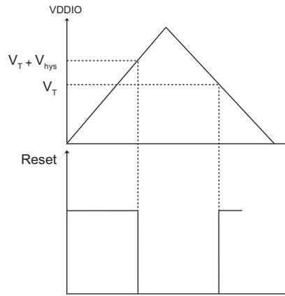
**Table 42-6. Backup Power Supply Zero-Power-on Reset Characteristics**
