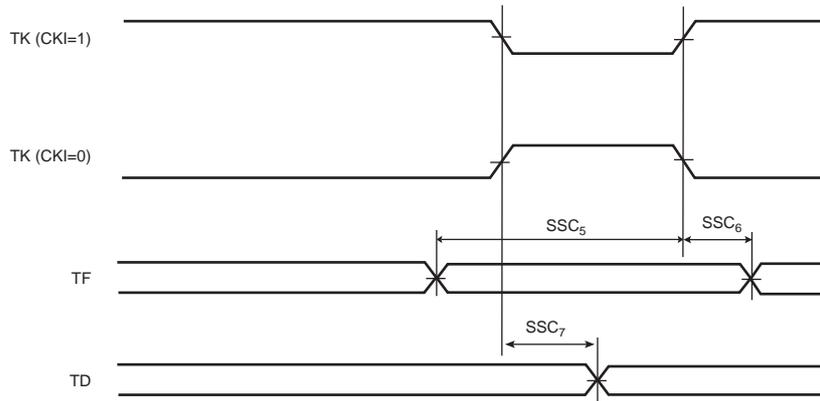
**Figure 42-25. SSC Receiver RK and RF as Input**
