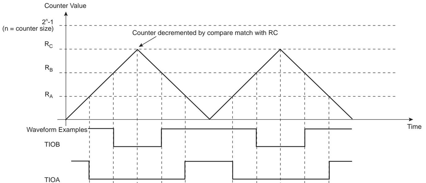
**Figure 35-14. WAVSEL = 11 with Trigger**
