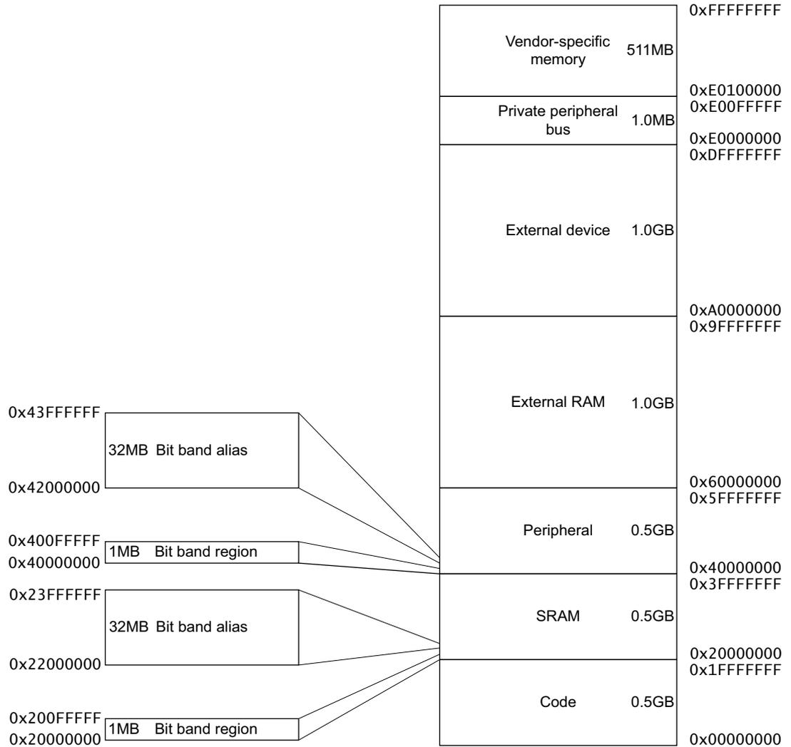
The regions for SRAM and peripherals include bit-band regions. Bit-banding provides atomic operations to bit data, see [“Bit-banding” on page 62](#).
