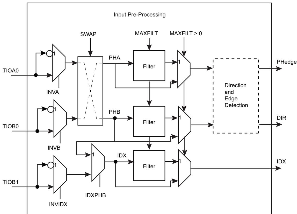
Input filtering can efficiently remove spurious pulses that might be generated by the presence of particulate contamination on the optical or magnetic disk of the rotary sensor.
