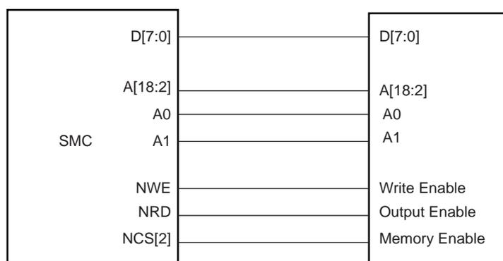
Figure 24-5. Memory Connection for a 16-bit Data Bus
