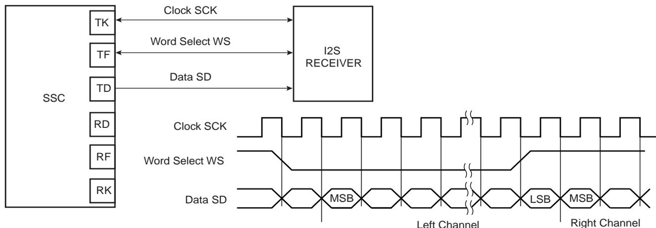
**Figure 30-18. Codec Application Block Diagram**
