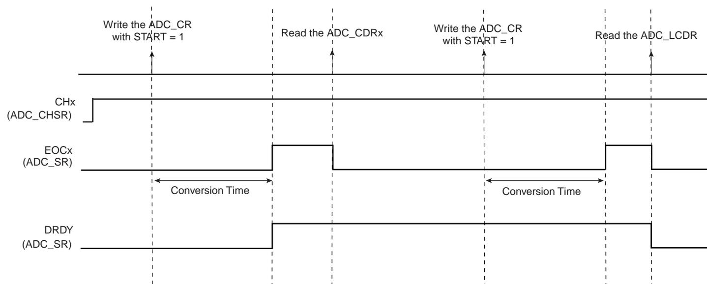
If the ADC12B\_CDR is not read before further incoming data is converted, the corresponding Overrun Error (OVRE) flag is set in the Status Register (ADC12B\_SR).
