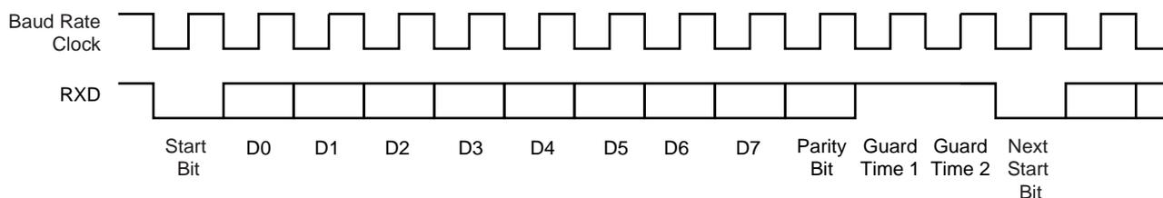
**Figure 34-32. T = 0 Protocol with Parity Error**
