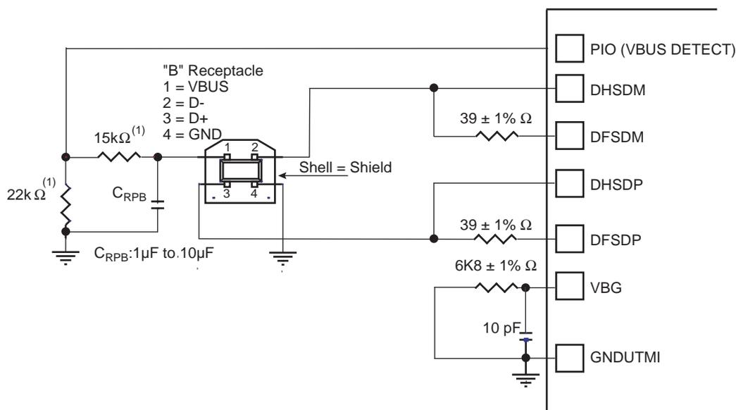
Note: The values shown on the 22 kΩ and 15 kΩ resistors are only valid with 3V3 supplied PIOs. Both 39 Ω resistors need to be placed as close to the device pins as possible.
