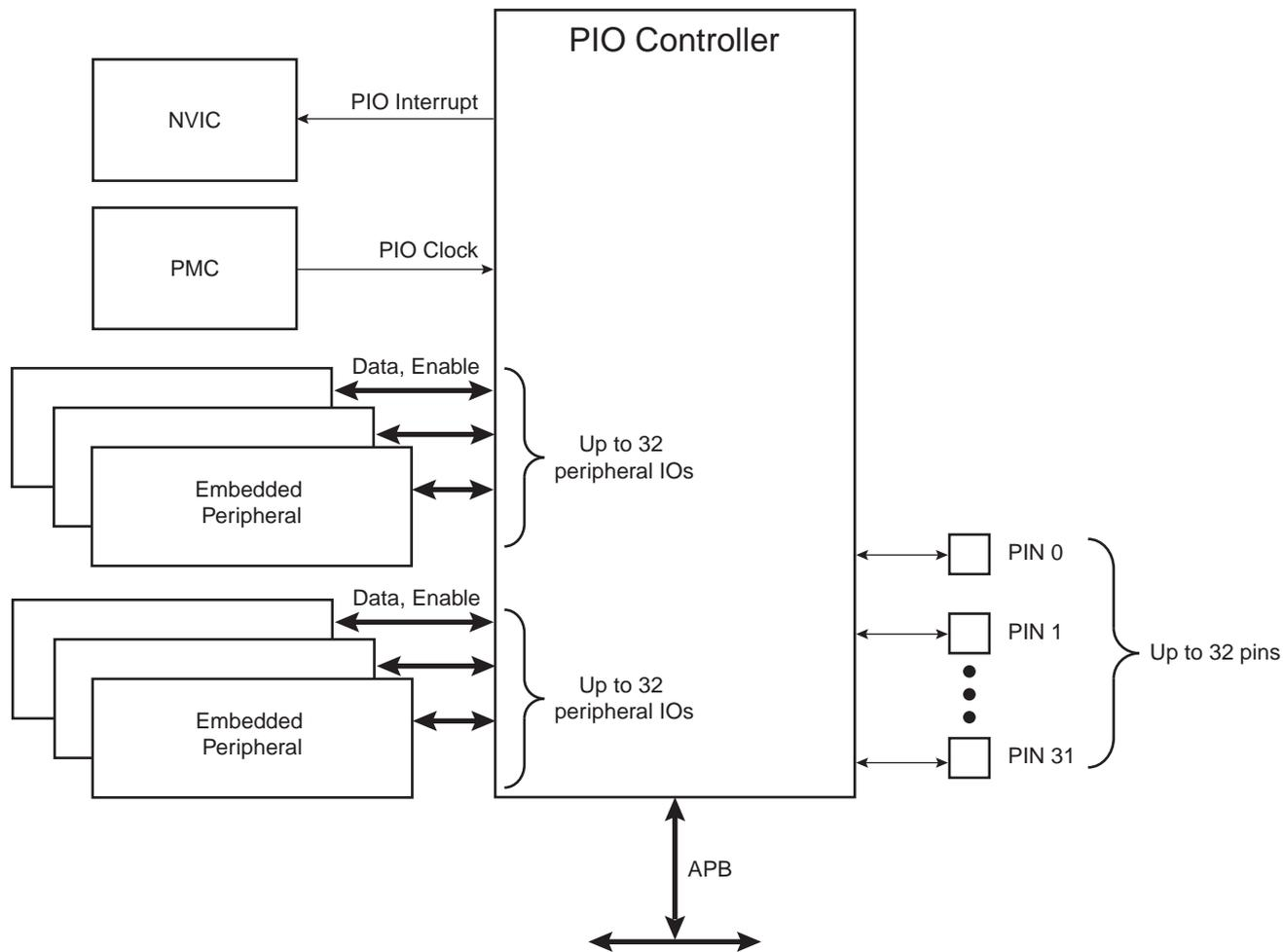
Figure 29-2. Application Block Diagram
