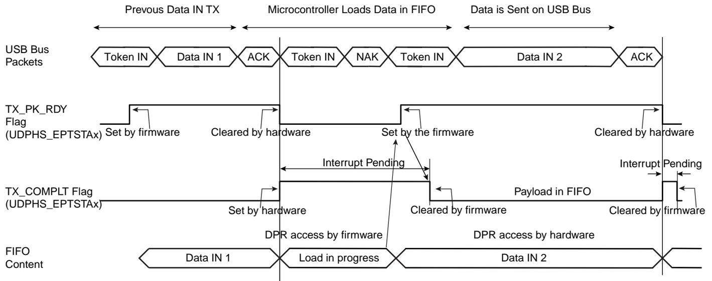
**Figure 38-9. Data IN Transfer for Endpoint with Two Banks**
