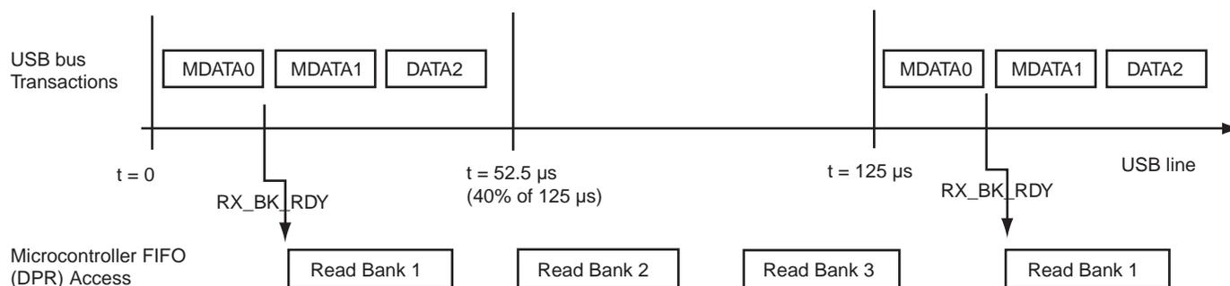
USB 2.0 supports individual High Speed isochronous endpoints that require data rates up to 192 Mb/s (24 MB/s): 3x1024 data bytes per microframe.
