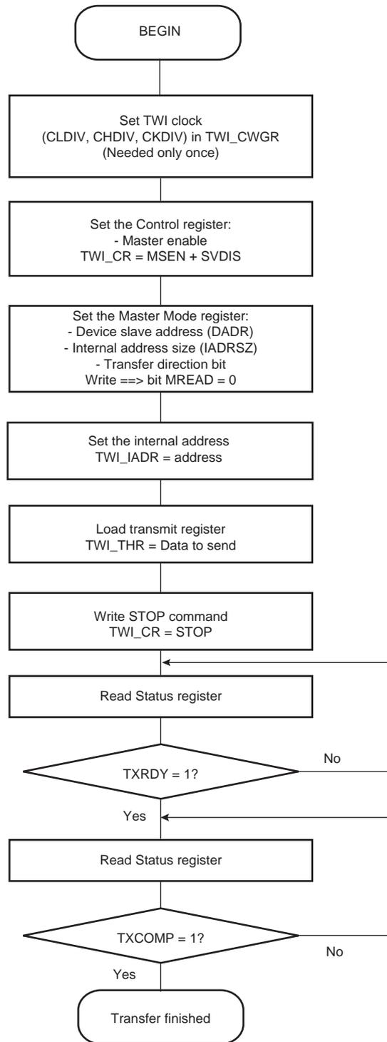
Figure 32-17. TWI Write Operation with Multiple Data Bytes with or without Internal Address
