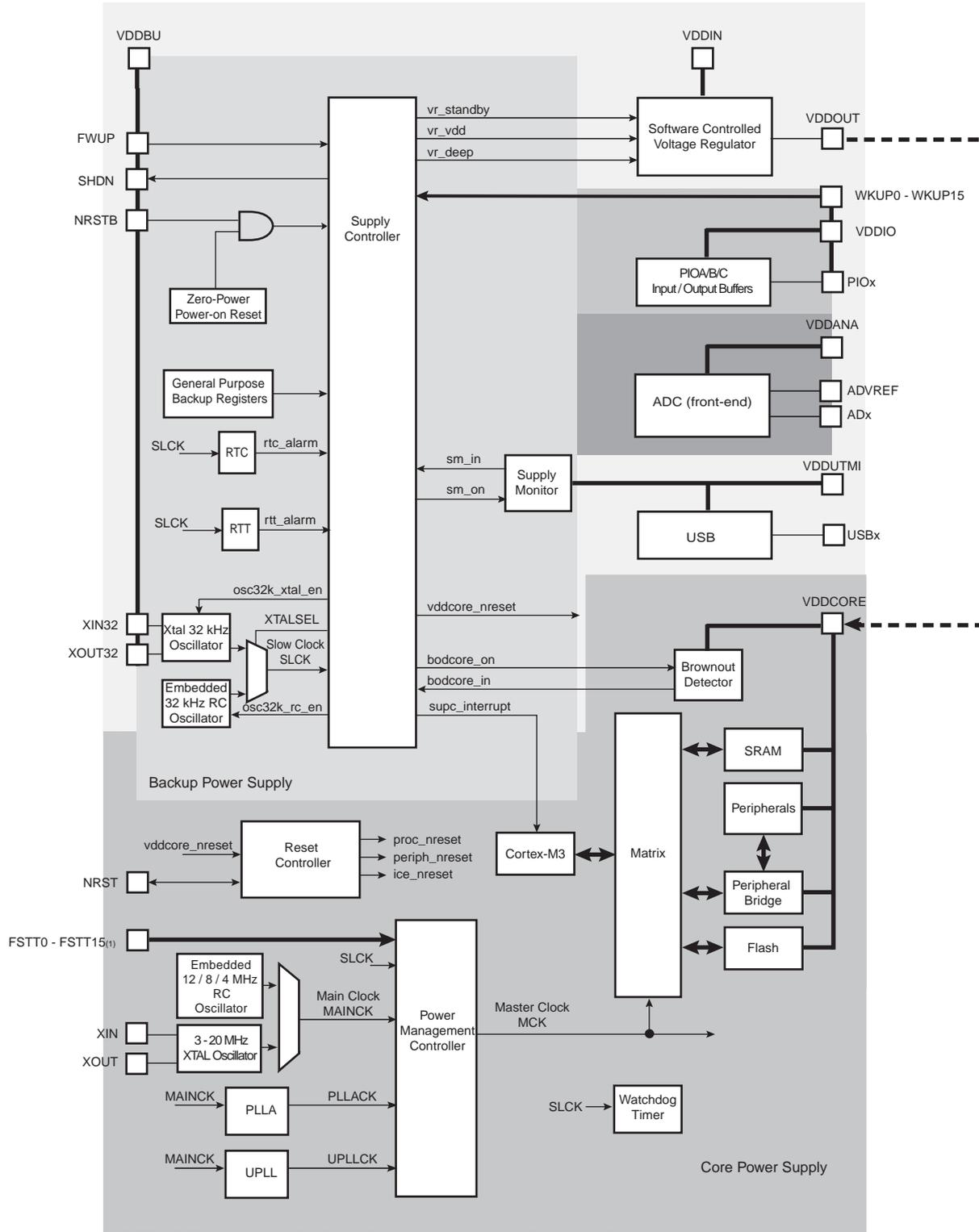
FSTT0 - FSTT15 are possible Fast Startup Sources, generated by WKUP0-WKUP15 Pins, but are not physical pins.
