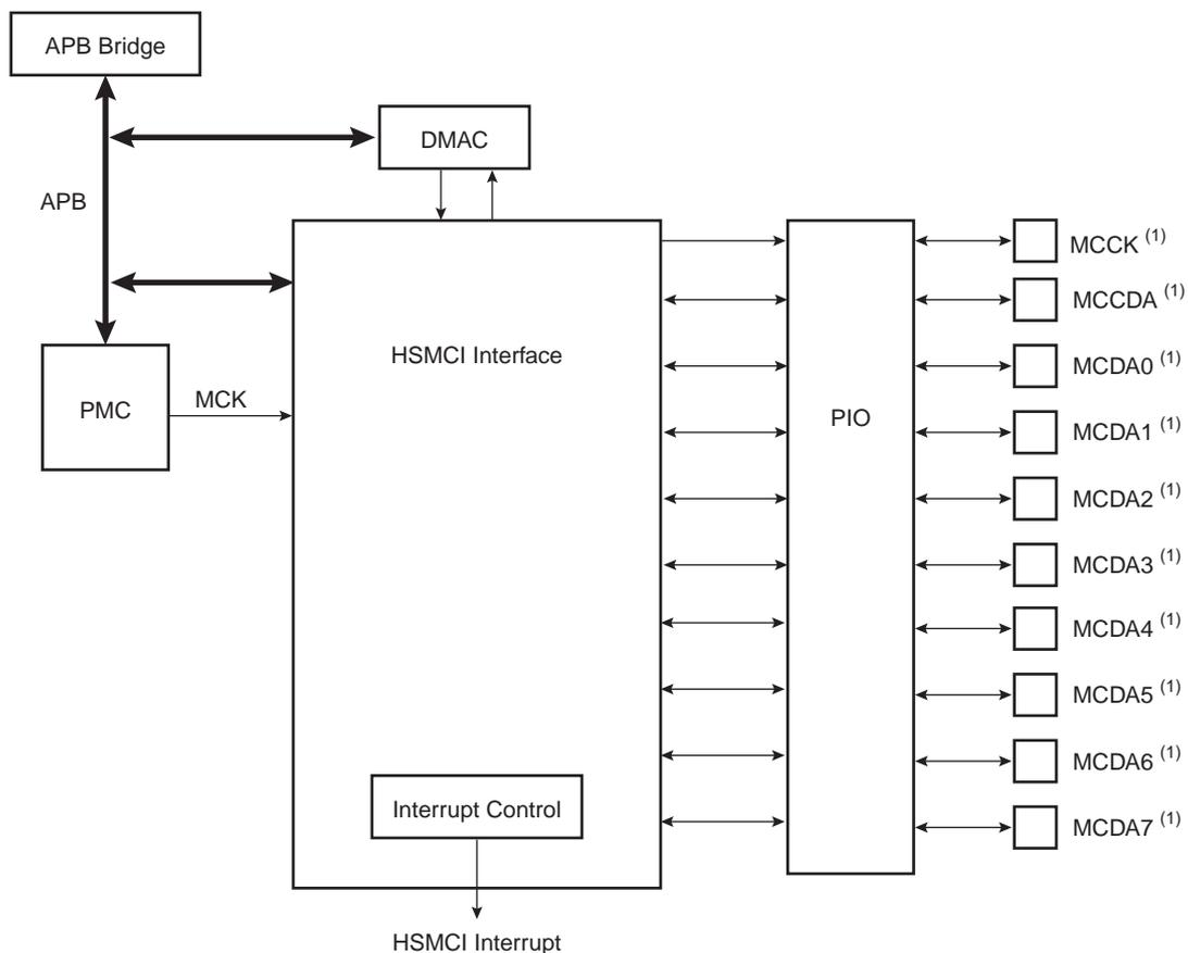
Note: 1. When several HSMCI (x HSMCI) are embedded in a product, MCCK refers to HSMCI<sub>x</sub>\_CK, MCCDA to HSMCI<sub>x</sub>\_CDA, MCDA<sub>y</sub> to HSMCI<sub>x</sub>\_DAY.
