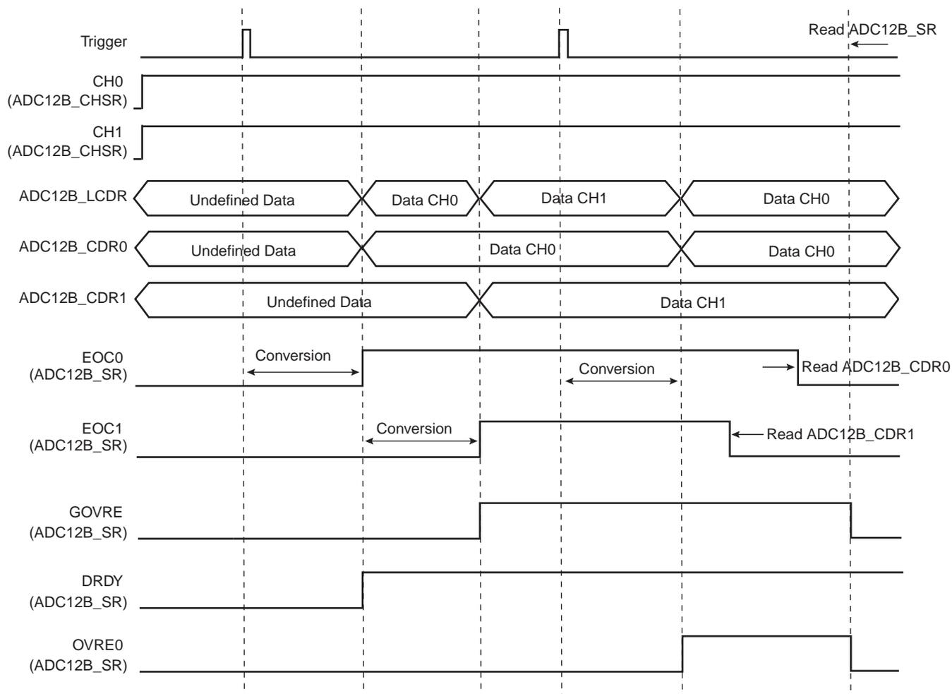
**Warning:** If the corresponding channel is disabled during a conversion or if it is disabled and then reenabled during a conversion, its associated data and its corresponding EOC and OVRE flags in ADC12B\_SR are unpredictable.
