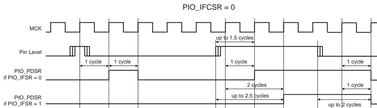
**Figure 29-6. Input Debouncing Filter Timing**
