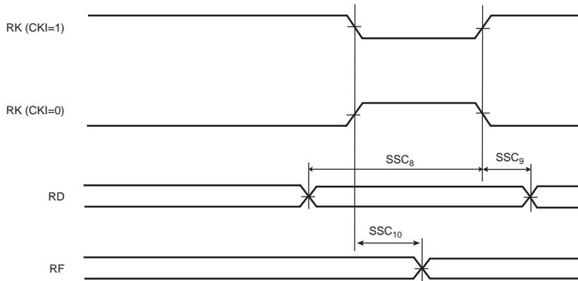
**Figure 42-27. SSC Receiver, RK and RF as Output**
