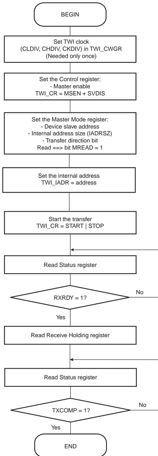
Figure 32-20. TWI Read Operation with Multiple Data Bytes with or without Internal Address
