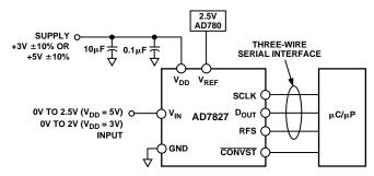
Figure 5. Typical Connection Diagram
