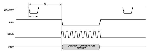
Figure 13. Mode 1 Operation Timing Diagram
