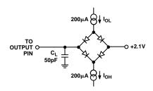
Figure 1. Load Circuit for Digital Output Timing Specifications
