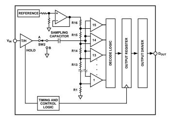
Figure 2. ADC Acquisition Phase
