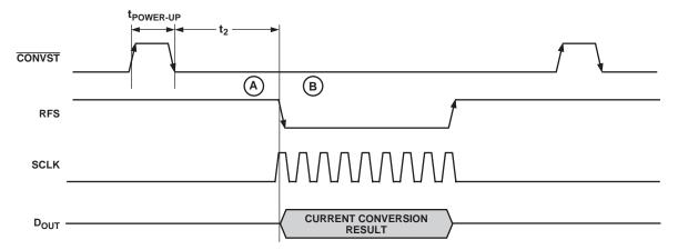
Figure 14. Mode 2 Operation Timing Diagram
