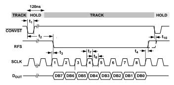
Figure 4. Track-and-Hold Timing
