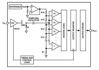
Figure 3. ADC Conversion Phase
