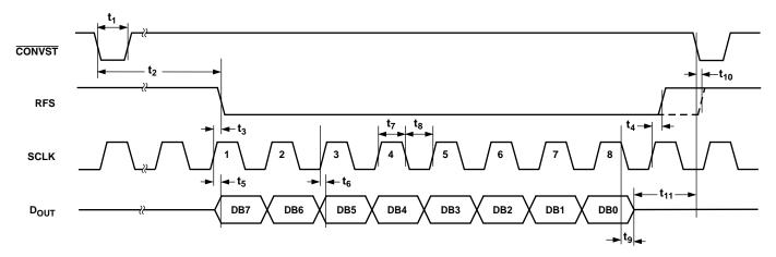
Figure 15. Serial Timing
