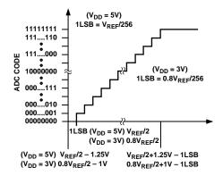
Figure 6. Transfer Characteristic
