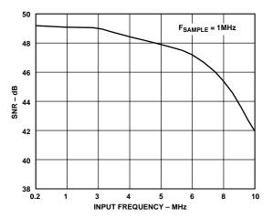
Figure 8. SNR vs. Input Frequency On the AD7827
