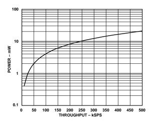
Figure 11. Power vs. Throughput
