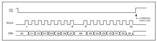
Figure 1. Serial interface timing diagram.
