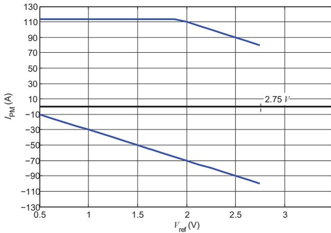
Figure 26: Measuring range versus external  $V_{ref}$  LXSR 25-NP
