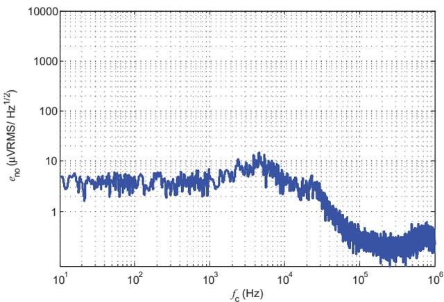
Figure 9: output noise voltage spectral density
