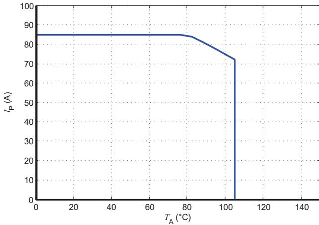
Figure 18:  $I_p$  vs  $T_A$  for LXSR 25-NPS
