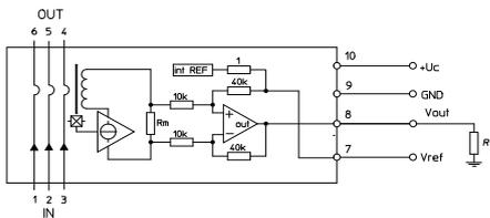
Figure 21: Test connection
