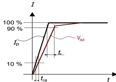
Figure 22: Response time  $t_r$  and reaction time  $t_{ra}$
