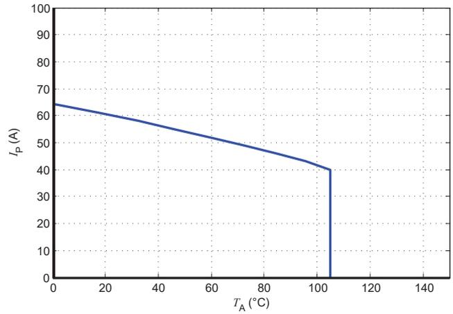
Figure 17:  $I_p$  vs  $T_A$  for LXSR 15-NPS
