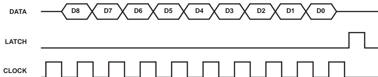
NOTE A: Data is clocked in on the positive leading edge of the clock. The latch should occur before the next positive leading edge of the clock. For definition of D0 to D8, see the control logic table.
