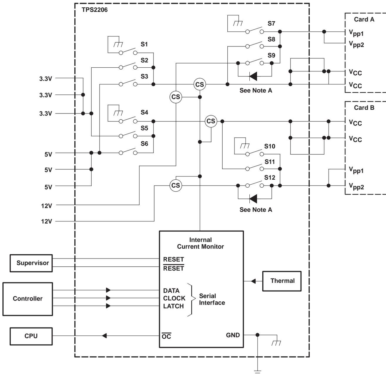
NOTE A: MOSFET switches S9 and S12 have a back-gate diode from the source to the drain. Unused switch inputs should never be grounded.
