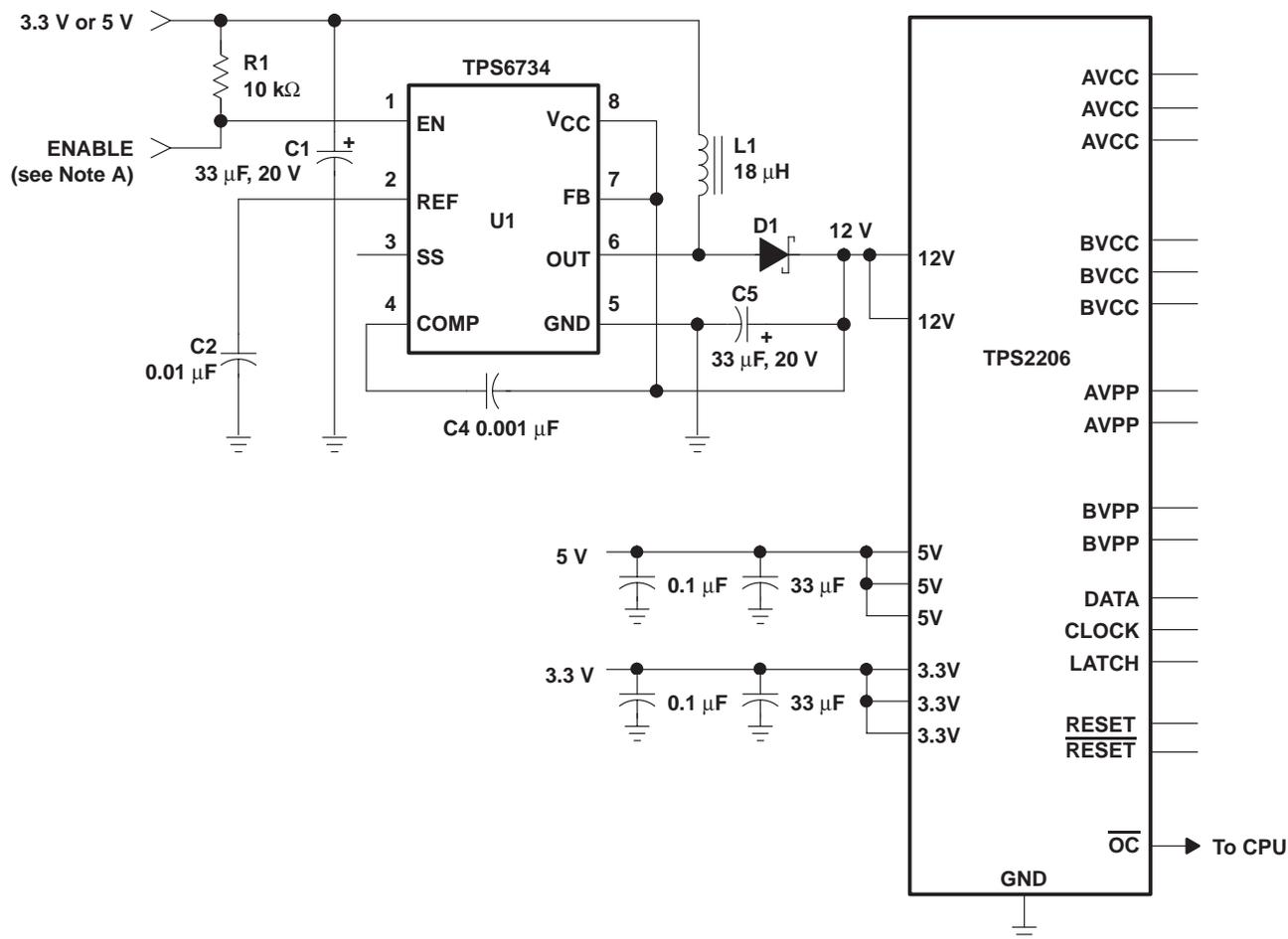
NOTE A: The enable terminal can be tied to a general purpose I/O terminal on the PCMCIA controller or tied high.
