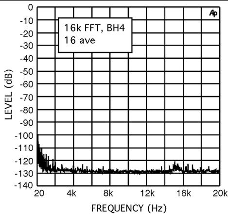
Figure 10. Line Out Noise Floor (Analog Loopthrough)
