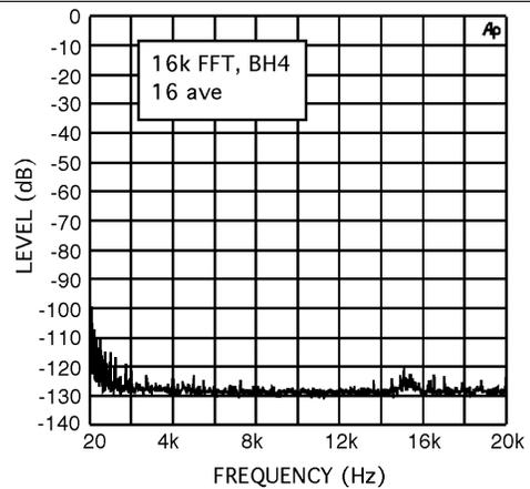
Figure 11. Line Level Out Noise Floor (Analog Loopthrough)
