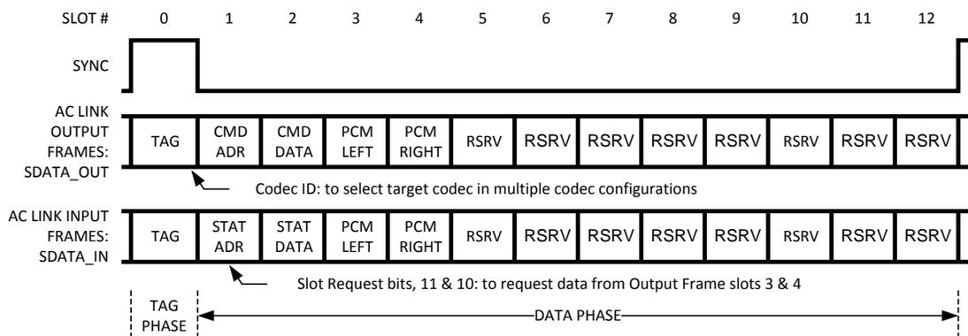
Figure 15. AC Link Bidirectional Audio Frame
