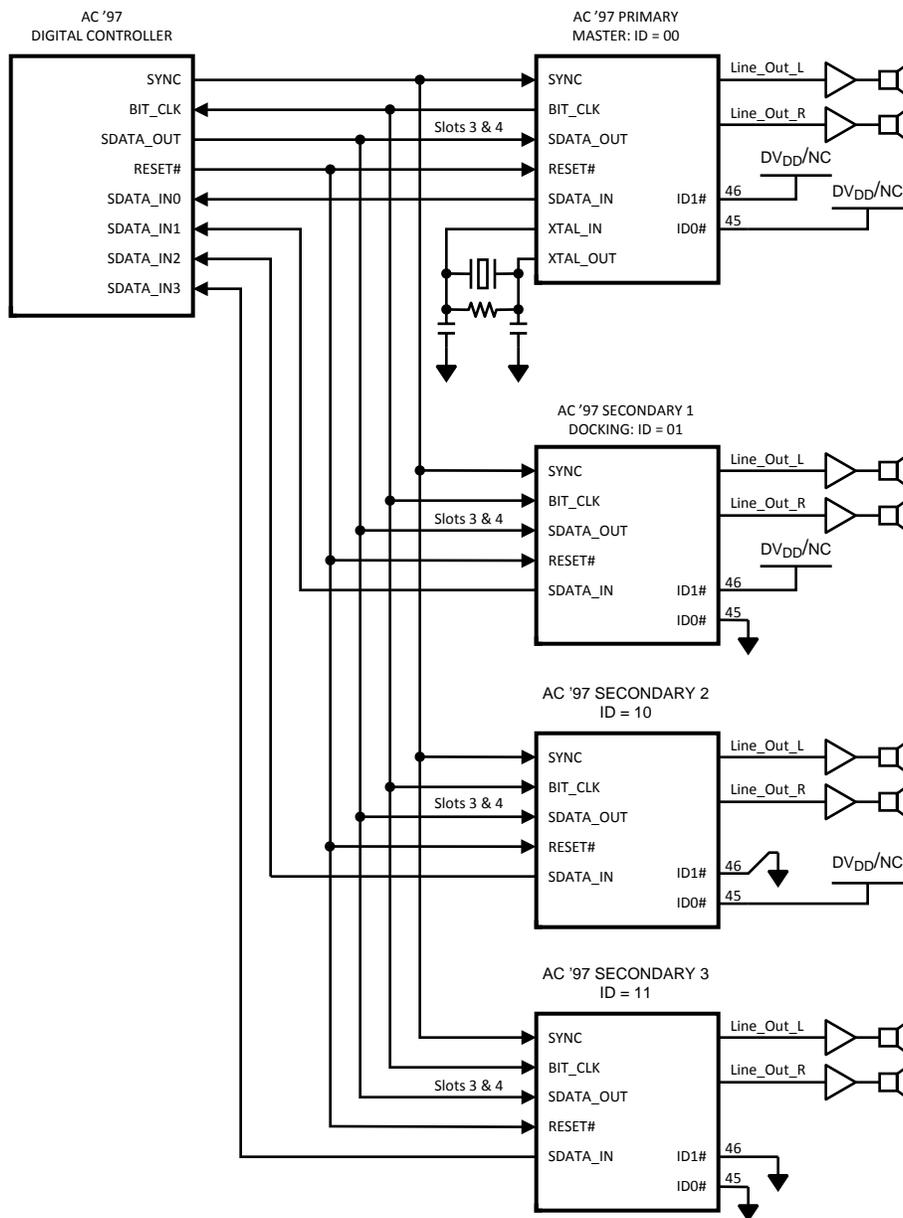
Figure 20. Multiple Codecs using Extended AC Link
