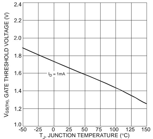
Fig. 6 Gate Threshold Variation vs. Junction Temperature
