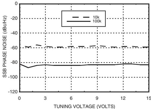
**Typical SSB Phase Noise @ Vtune = +12V**
