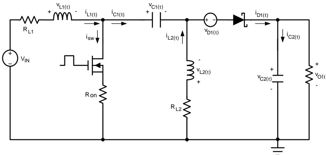
Using inductor volt-second balance & capacitor charge balance, the following equations are derived:
