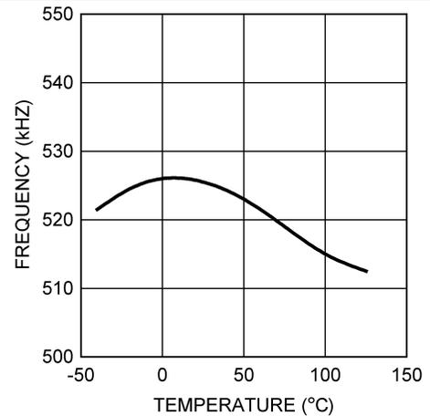
Figure 4. Oscillator Frequency vs Temperature - "Y"
