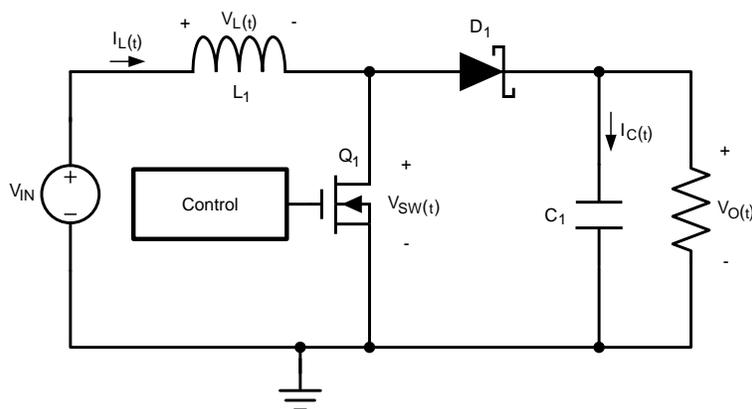
**Figure 13. Simplified Schematic**
