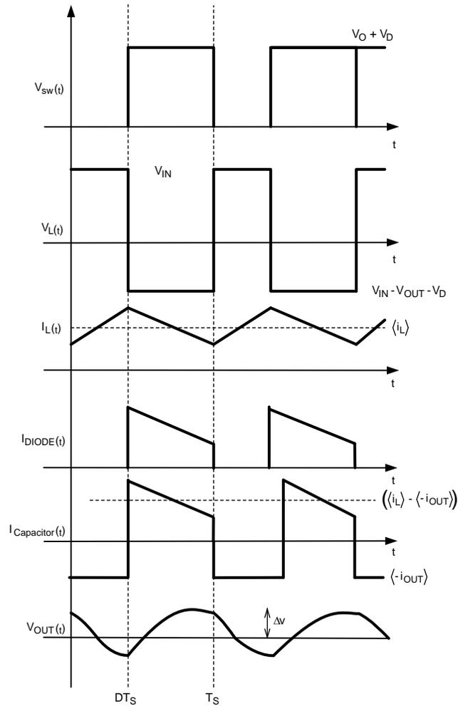
**Figure 14. Typical Waveforms**
