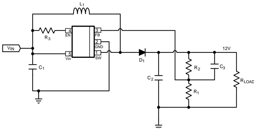
Figure 18. LM2735X (1.6 MHz):  $V_{IN} = 5$  V,  $V_{OUT} = 12$  V @ 350 mA
