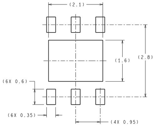
DIMENSIONS ARE IN MILLIMETERS
