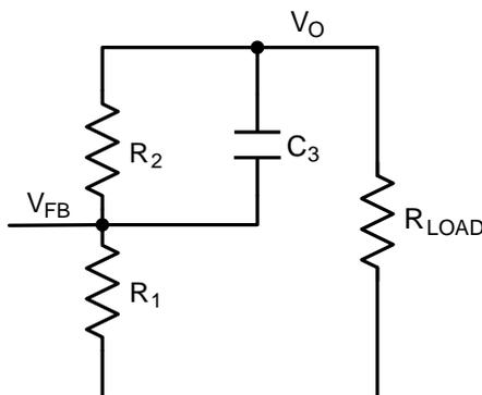
**Figure 20. Setting V<sub>out</sub>**
