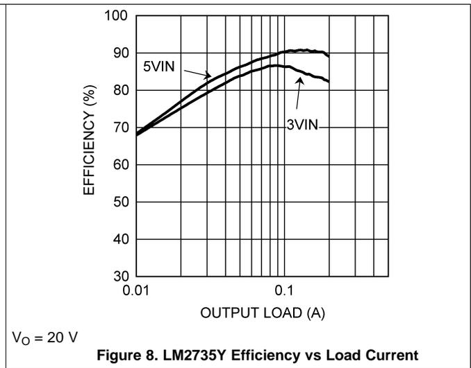
Figure 8. LM2735Y Efficiency vs Load Current
