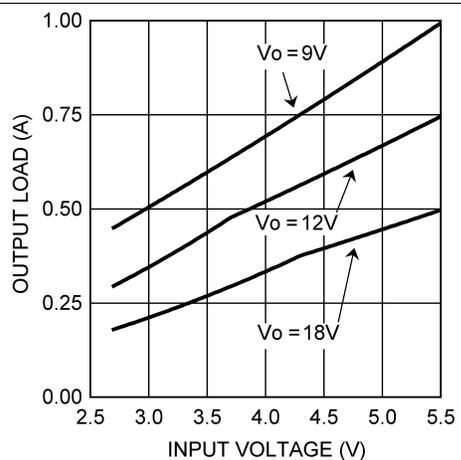
Figure 5. Typical Maximum Output Current vs  $V_{IN}$
