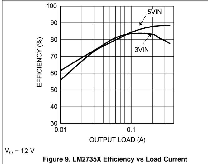
Figure 9. LM2735X Efficiency vs Load Current
