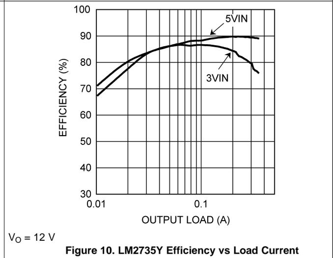
Figure 10. LM2735Y Efficiency vs Load Current
