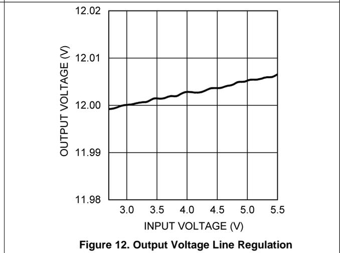
Figure 12. Output Voltage Line Regulation
