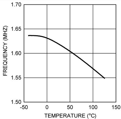
Figure 3. Oscillator Frequency vs Temperature - "X"
