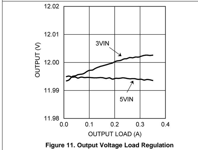
Figure 11. Output Voltage Load Regulation
