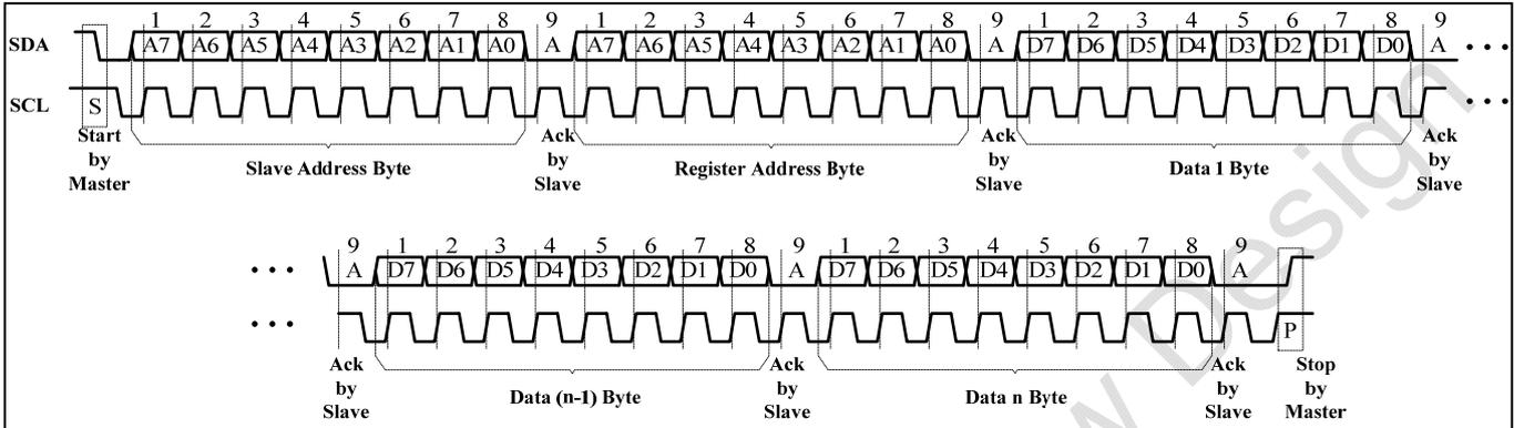
Figure 5 Writing to IS31FL3236 (Automatic Address Increment)
