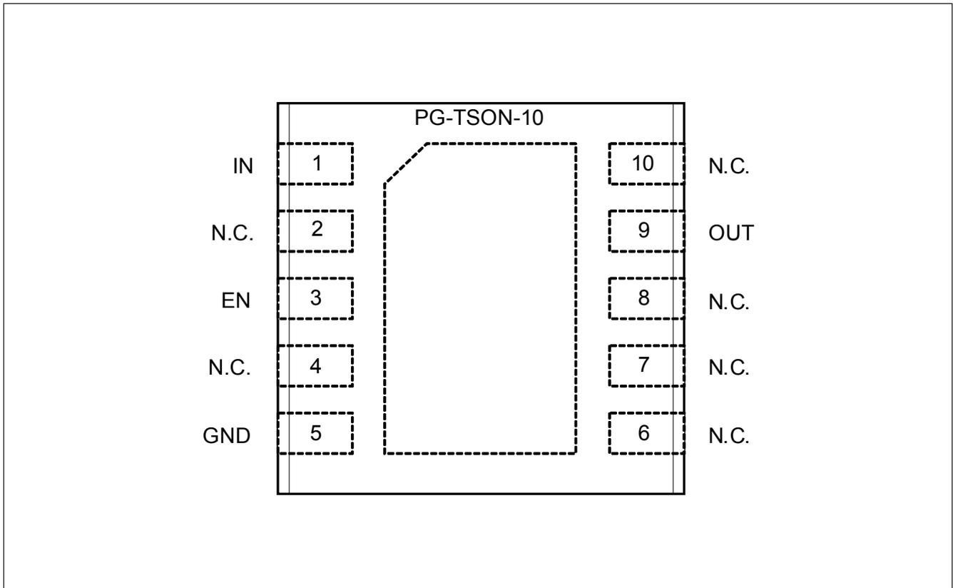
Figure 2 Pin Configuration IFX30081LDV33 in PG-TSON-10 package
