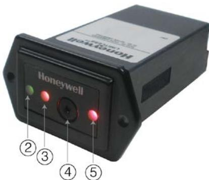
**NOTE:** Use a blunt object, such as a paper clip or tooth pick to actuate the function switch ④.
