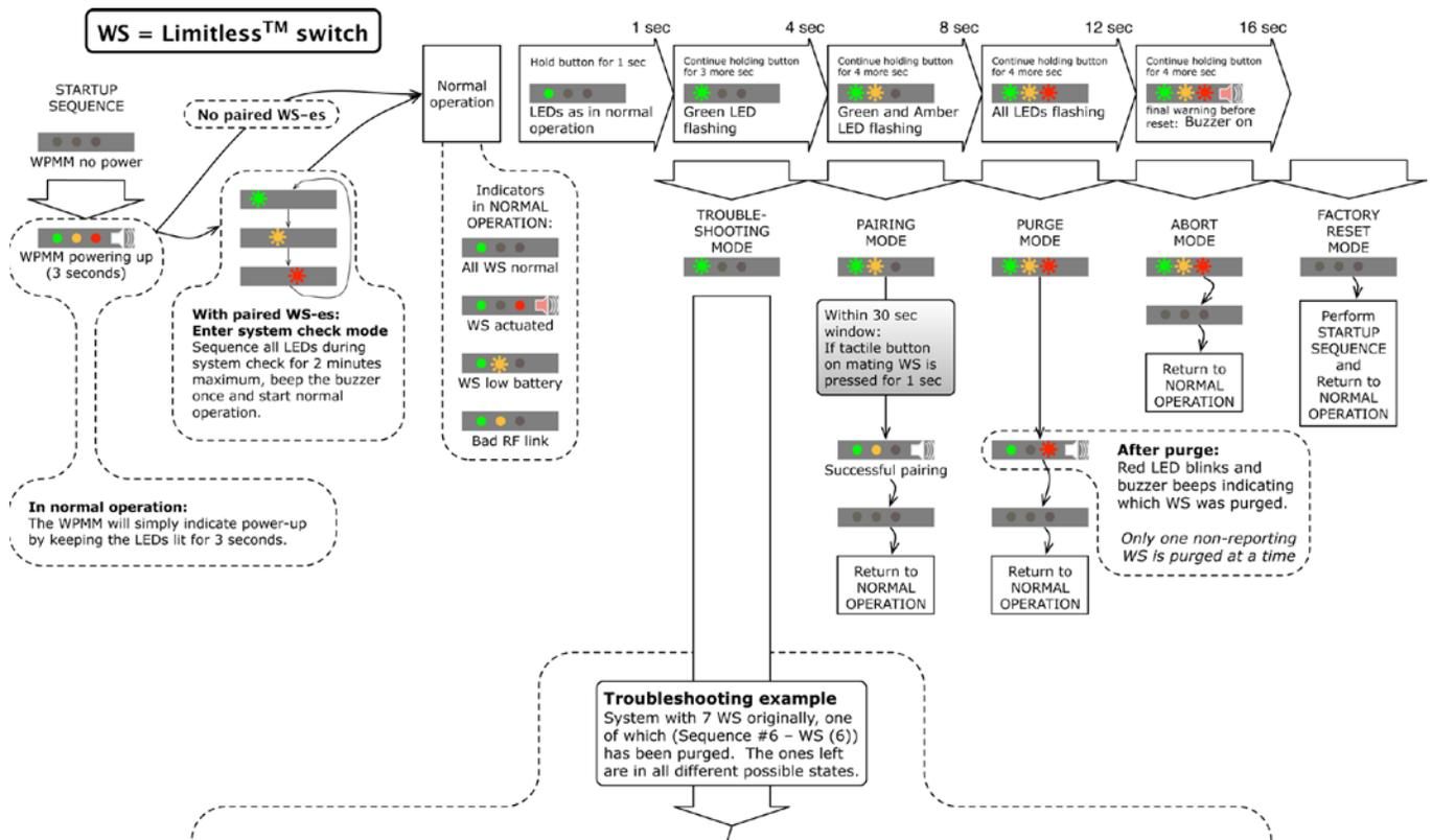
Figure 9. WPMM Operation and LED Functions Chart – part 2
