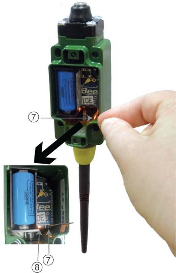
**NOTE:** Use a blunt object, such as a paper clip or tooth pick to actuate the function switch ⑦.
