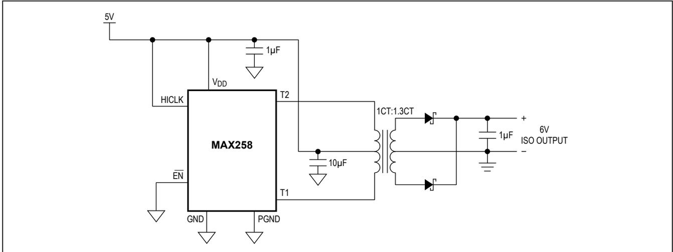
Figure 3. 5V to Isolated, Unregulated 6V Application Circuit
