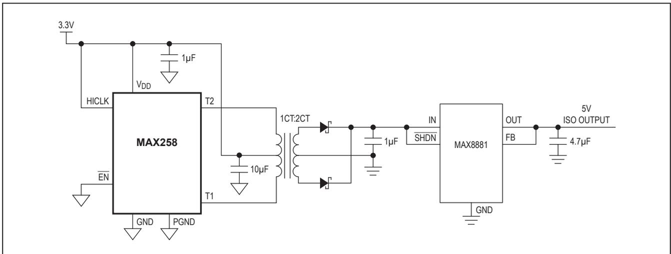
Figure 4. 3.3V to Isolated, Regulated 5V Application Circuit
