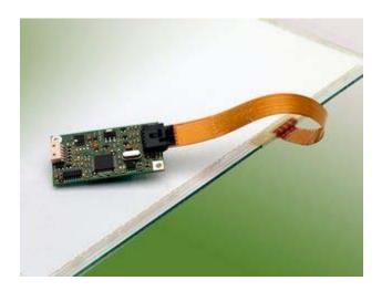
$3M^{TM}$  Touch Systems has more than 25 years of surface capacitive technology expertise and specifically designed the  $3M^{TM}$  MicroTouch $^{TM}$  System SCT3250EX to meet the performance requirements of display applications ranging from 5.7 to 32 inches. As an all-glass design, the SCT3250EX touch system offers light transmission up to 11.5% better than typical resistive sensors and 3.5% better than typical surface capacitive sensors (based on published specifications).
