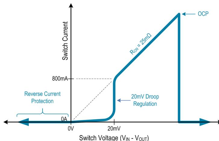
Figure 7. “Ideal Diode” Reverse-Current Protection V-I Curve
