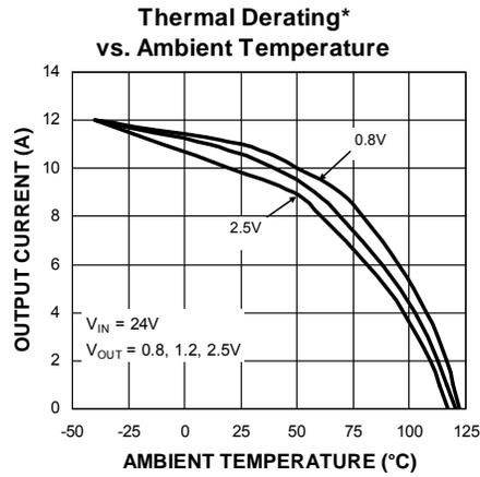
**Die Temperature\*** : The temperature measurement was taken at the hottest point on the MIC26901 case mounted on a 5 square inch 4 layer, 0.62", FR-4 PCB with 2oz finish copper weight per layer, see Thermal Measurement section. Actual results will depend upon the size of the PCB, ambient temperature and proximity to other heat emitting components.
