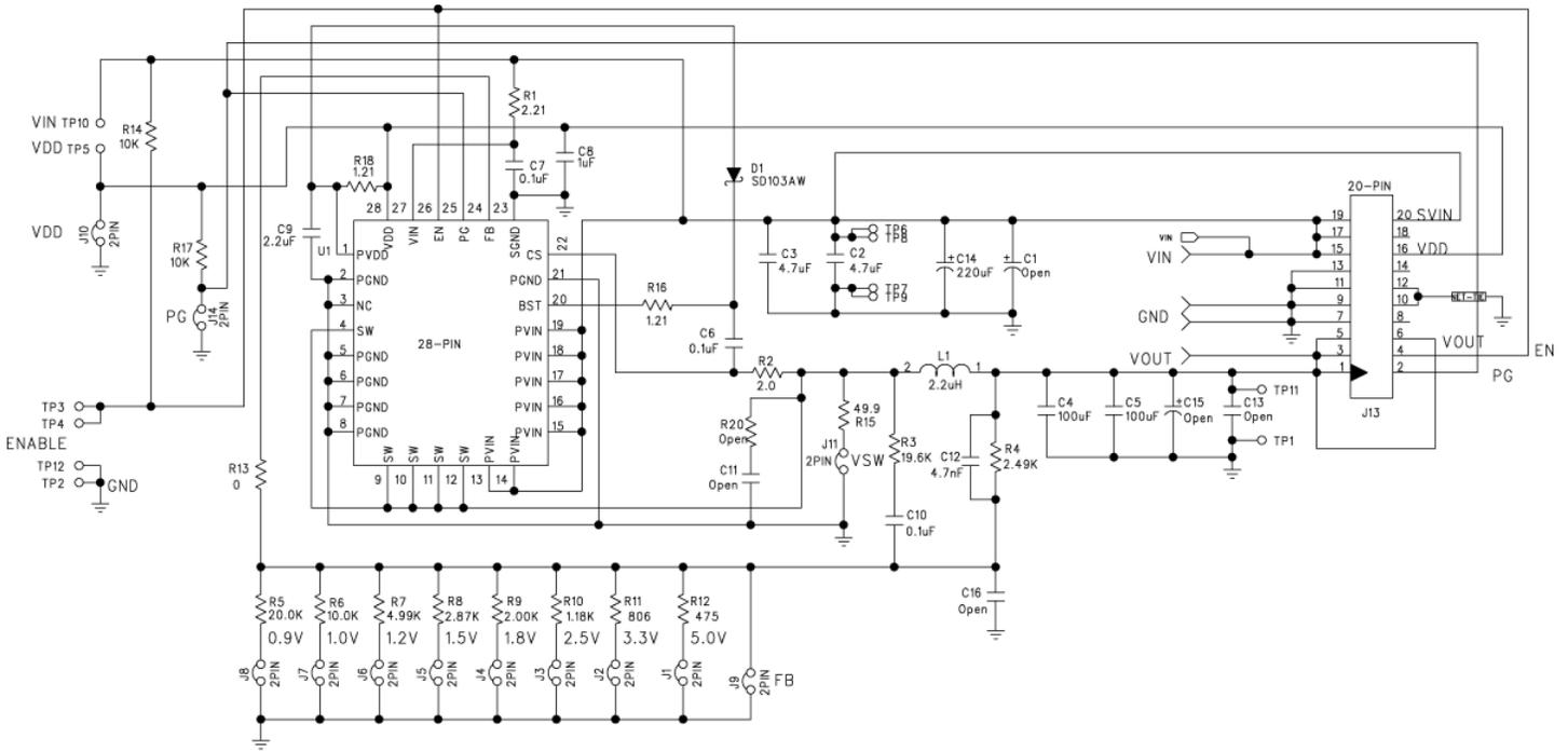
**Figure 8. Schematic of MIC26901 Evaluation Board**
