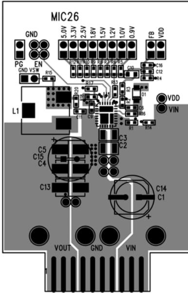
Figure 9. MIC26901 Evaluation Board Top Layer
