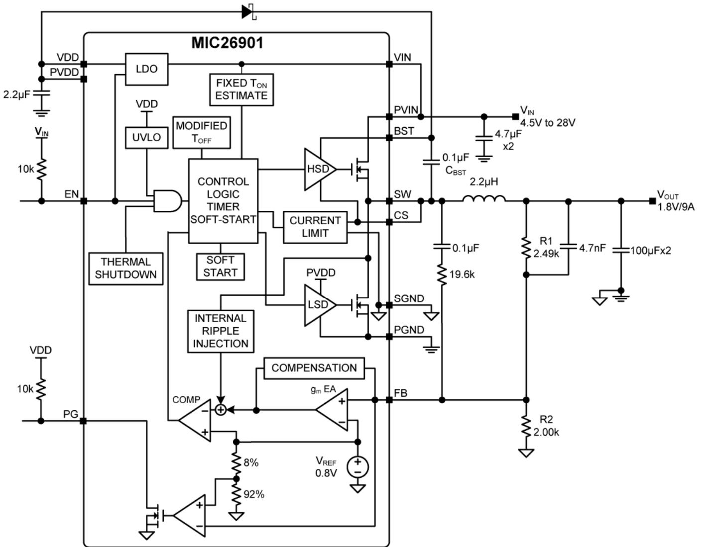
Figure 1. MIC26901 Block Diagram
