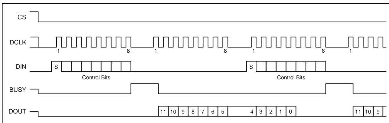
**Figure 11. Conversion Timing, 16 Clocks-per-Conversion, 8-Bit Bus Interface.
