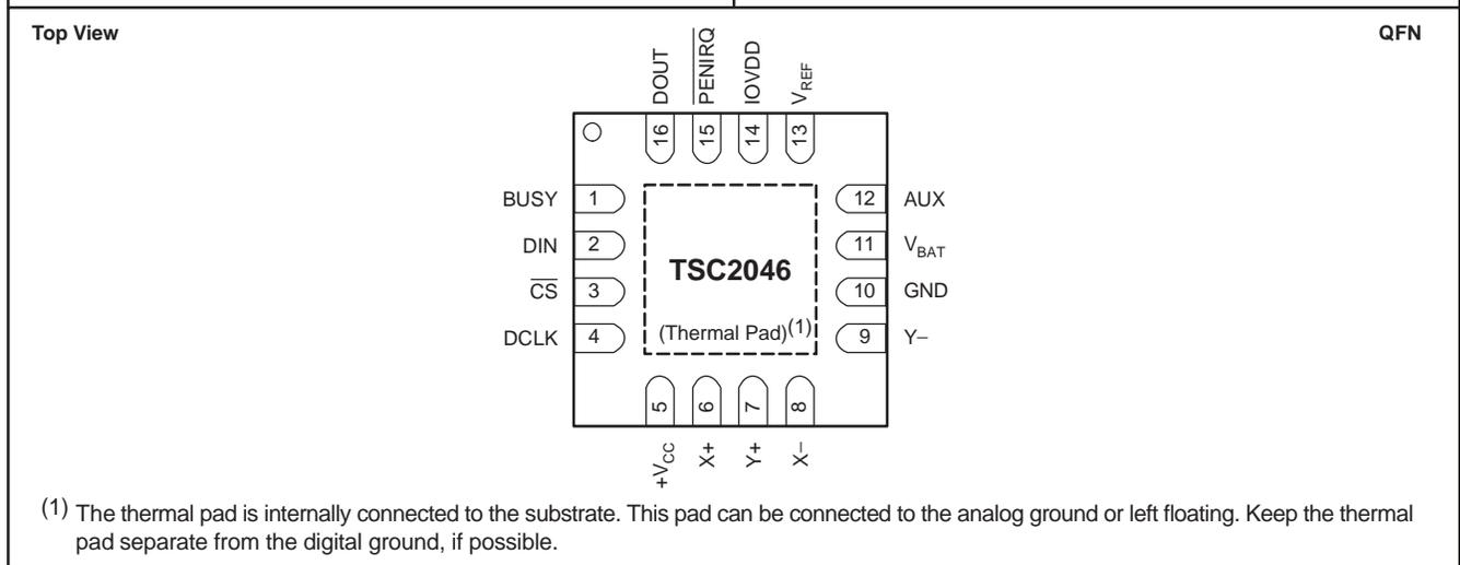
(1) The thermal pad is internally connected to the substrate. This pad can be connected to the analog ground or left floating. Keep the thermal pad separate from the digital ground, if possible.
