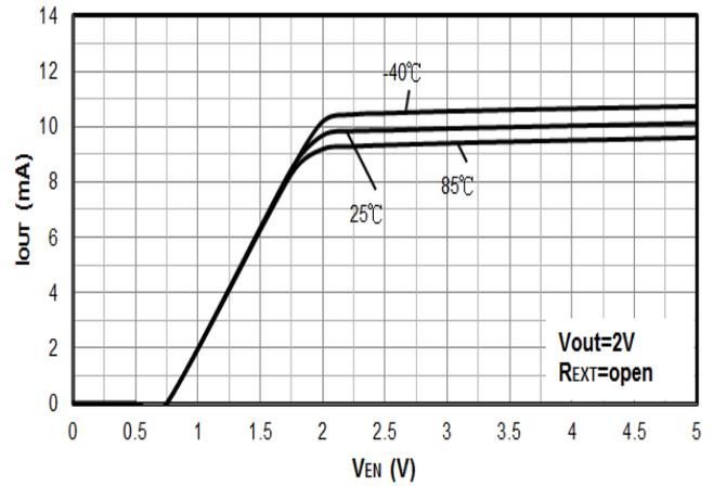
**Figure 13.  $V_{EN}$  vs.  $I_{OUT}$  ( $R_{EXT}=open$ )**
