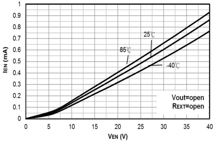
**Figure 7.  $V_{EN}$  vs.  $I_{EN}$  ( $R_{EXT}=open$ )**
