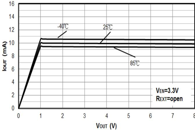
**Figure 10.  $V_{OUT}$  vs.  $I_{OUT}$  ( $R_{EXT}=open$ )**
