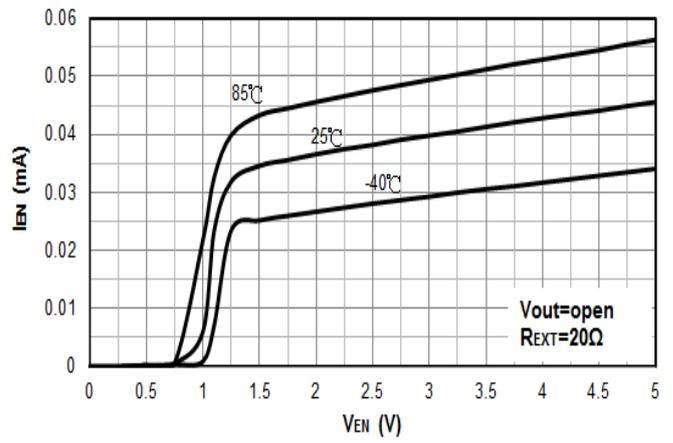
**Figure 17.  $V_{EN}$  vs.  $I_{EN}$  ( $R_{EXT}=20\Omega$ )**
