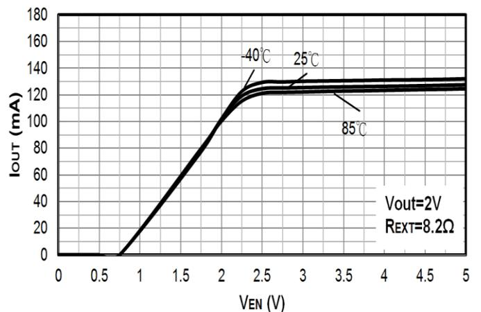
**Figure 15.  $V_{EN}$  vs.  $I_{OUT}$  ( $R_{EXT}=8.2\Omega$ )**
