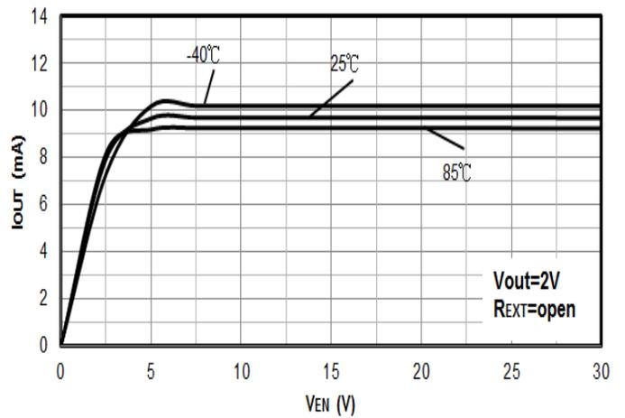
**Figure 4.  $V_{EN}$  vs.  $I_{OUT}$  ( $R_{EXT}=open$ )**
