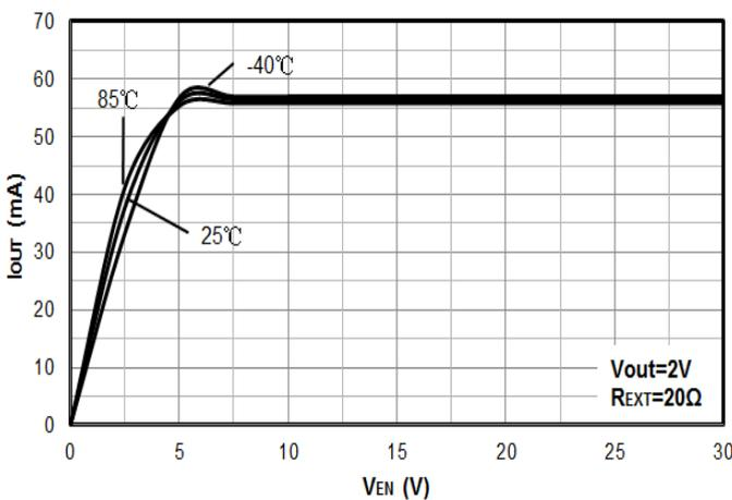
**Figure 5.  $V_{EN}$  vs.  $I_{OUT}$  ( $R_{EXT}=20\Omega$ )**
