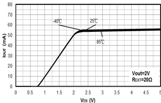
**Figure 14.  $V_{EN}$  vs.  $I_{OUT}$  ( $R_{EXT}=20\Omega$ )**
