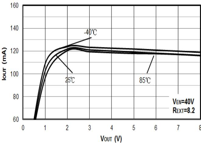
**Figure 3.  $V_{OUT}$  vs.  $I_{OUT}$  ( $R_{EXT}=8.2\Omega$ )**
