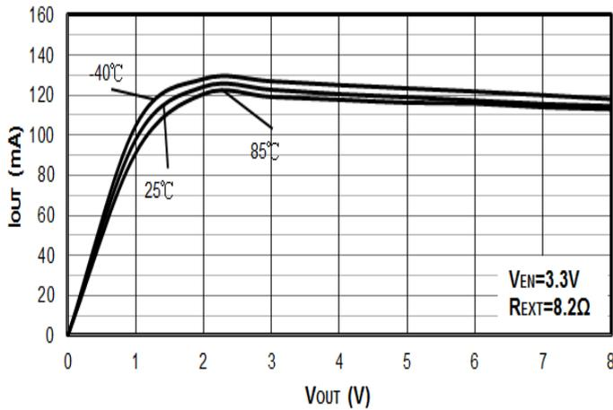
**Figure 12.  $V_{OUT}$  vs.  $I_{OUT}$  ( $R_{EXT}=8.2\Omega$ )**
