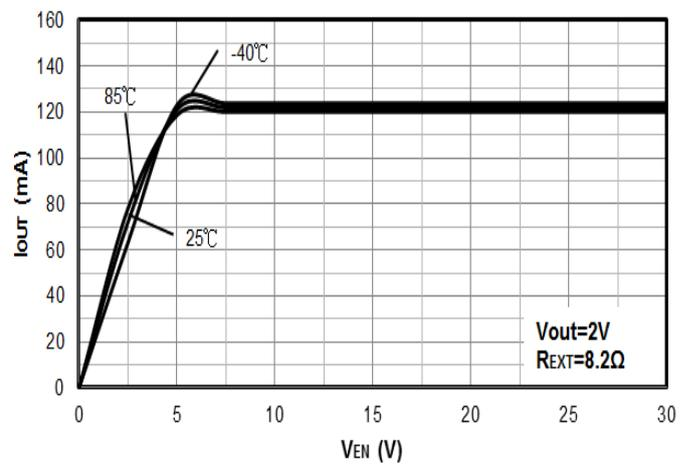
**Figure 6.  $V_{EN}$  vs.  $I_{OUT}$  ( $R_{EXT}=8.2\Omega$ )**
