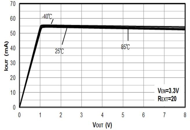
**Figure 11.  $V_{OUT}$  vs.  $I_{OUT}$  ( $R_{EXT}=20\Omega$ )**
