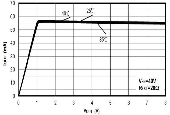
**Figure 2.  $V_{OUT}$  vs.  $I_{OUT}$  ( $R_{EXT}=20\Omega$ )**
