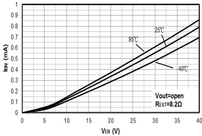
**Figure 9.  $V_{EN}$  vs.  $I_{EN}$  ( $R_{EXT}=8.2\Omega$ )**
