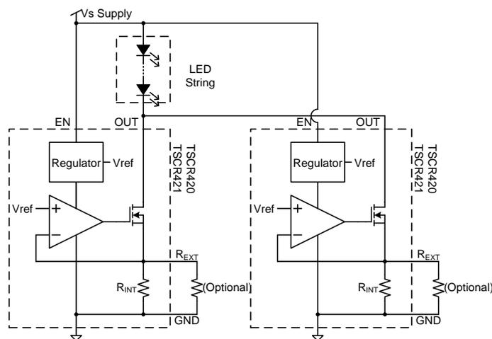
**Figure 21: Application Circuit for Increasing LED Current**
