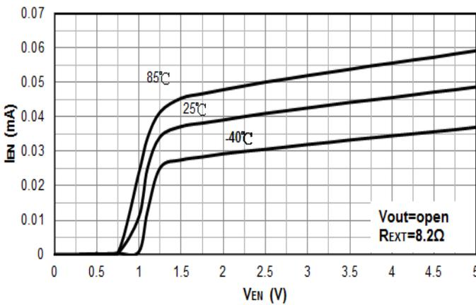
**Figure 18.  $V_{EN}$  vs.  $I_{EN}$  ( $R_{EXT}=8.2\Omega$ )**
