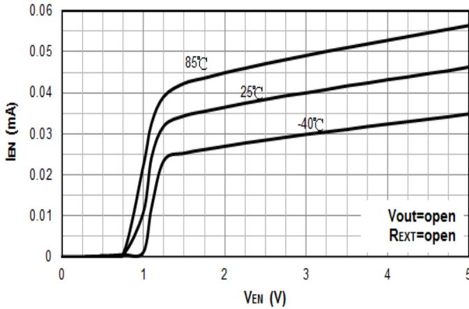
**Figure 16.  $V_{EN}$  vs.  $I_{EN}$  ( $R_{EXT}=open$ )**
