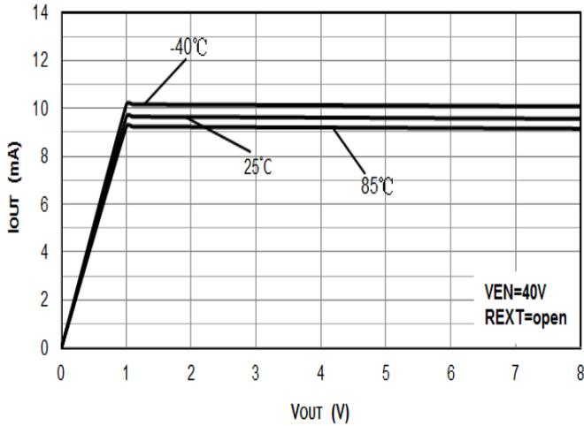
**Figure 1.  $V_{OUT}$  vs.  $I_{OUT}$  ( $R_{EXT}=open$ )**
