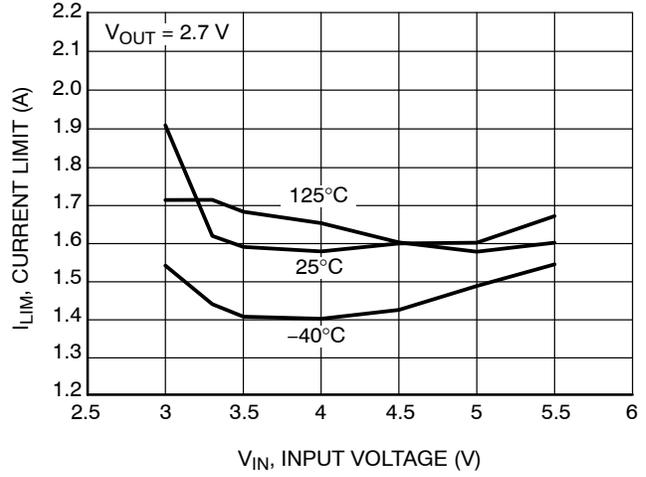
Figure 12. Peak Current Limit vs. Input Voltage
