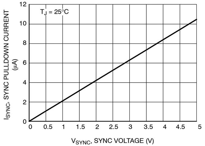
Figure 4. Sync Pulldown Current vs. Sync Voltage
