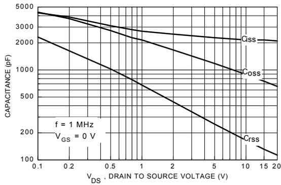
**Figure 9. Capacitance Characteristics.**
