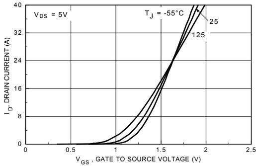
Figure 5. Transfer Characteristics.
