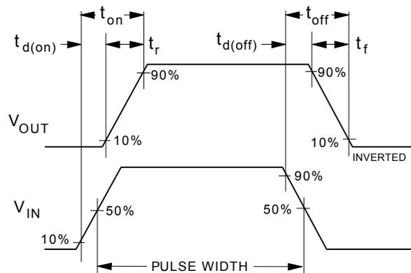
**Figure 12. Switching Waveforms.**
