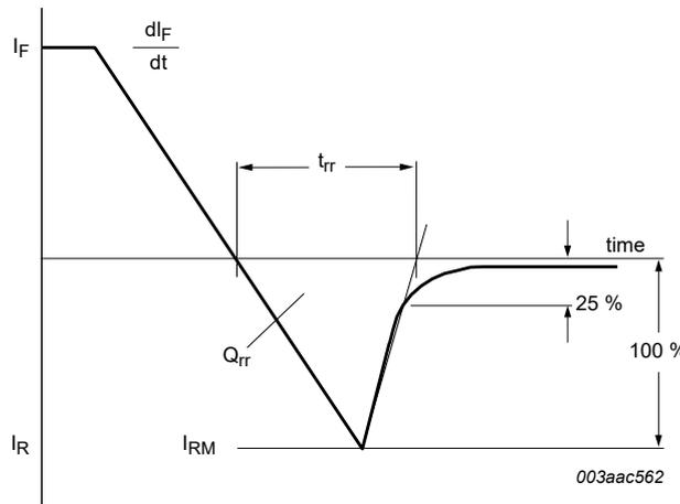
Fig. 15. Reverse recovery definition; ramp recovery
