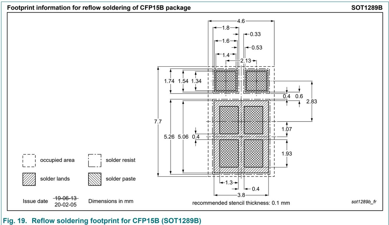
Fig. 19. Reflow soldering footprint for CFP15B (SOT1289B)
