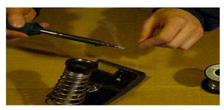
**Step 4: Clean the Soldering Tip**
