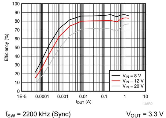
Figure 6-4. Efficiency vs Load Current
