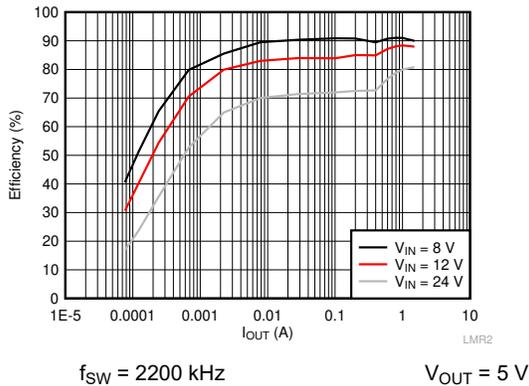
Figure 6-3. Efficiency vs Load Current
