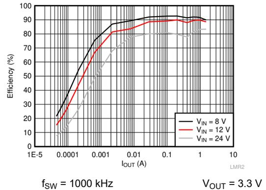
Figure 6-2. Efficiency vs Load Current
