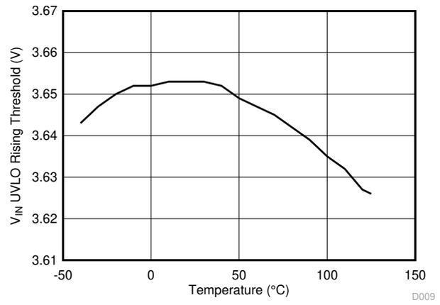
**Figure 6-10.  $V_{IN}$  UVLO Rising Threshold vs Junction Temperature**
