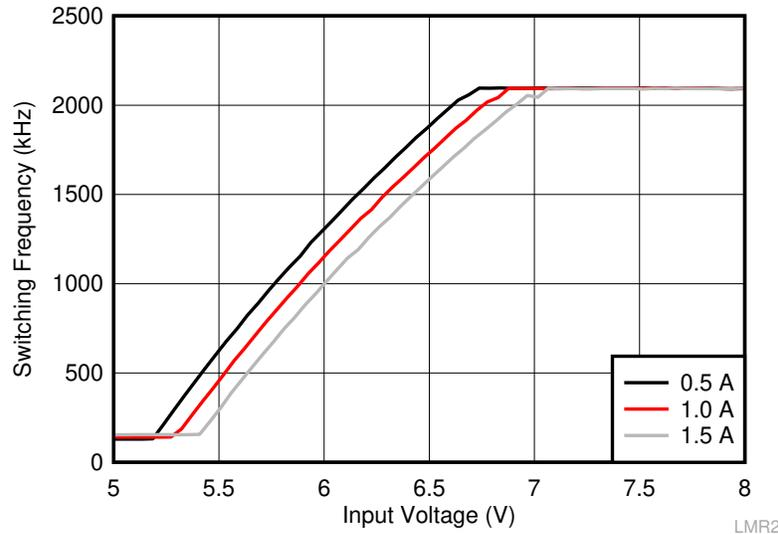
Figure 7-8. Frequency Foldback at Dropout ( $V_{OUT} = 5\text{ V}$ ,  $f_{SW} = 2100\text{ kHz}$ )
