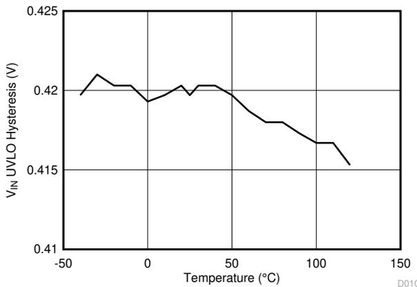
**Figure 6-11.  $V_{IN}$  UVLO Hysteresis vs Junction Temperature**
