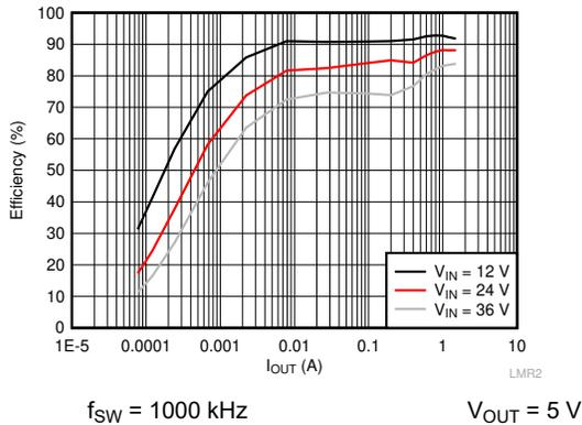
Figure 6-1. Efficiency vs Load Current
