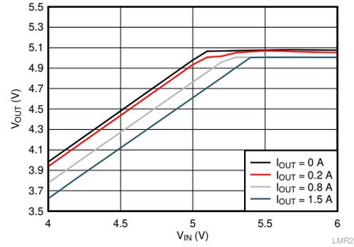
$f_{SW} = 2200 \text{ kHz}$   $V_{OUT} = 5 \text{ V}$
