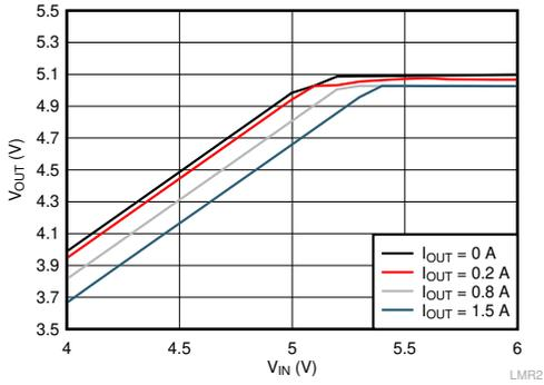
$f_{SW} = 1000 \text{ kHz}$   $V_{OUT} = 5 \text{ V}$
