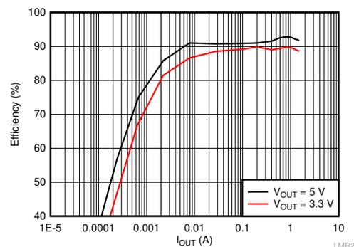
**Efficiency vs Load,  $V_{IN} = 12\text{ V}$**
