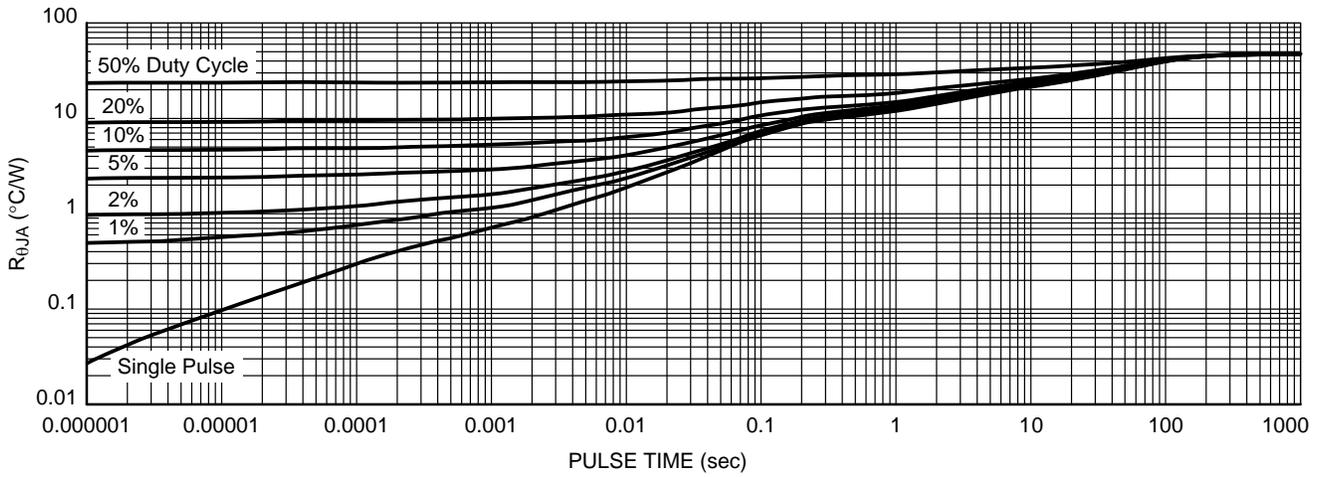
Figure 13. Thermal Characteristics
