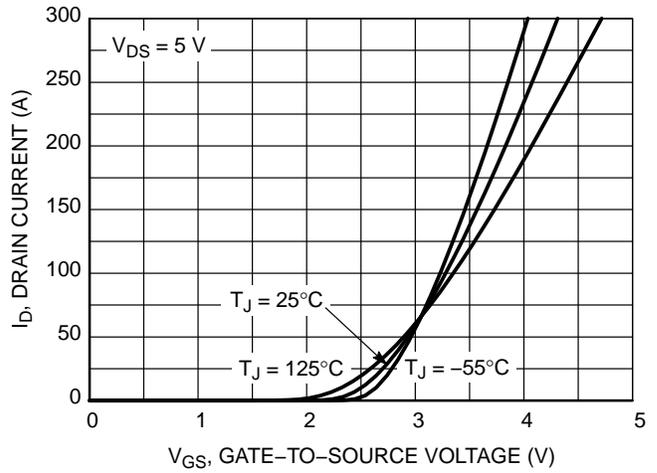
Figure 2. Transfer Characteristics
