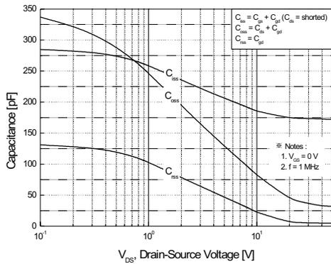
Figure 5. Capacitance Characteristics
