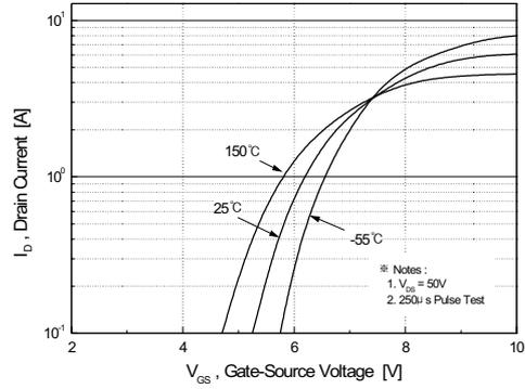
Figure 2. Transfer Characteristics
