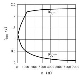
$\begin{array}{c} \text{R}_{L} \ (\Omega) \\ \text{Figure 9. Typical DS90LV031, D}_{0} \ \text{vs R}_{L}, \\ \text{V}_{CC} = 3.3 \text{V, T}_{A} = 25 ^{\circ} \text{C} \end{array}$
