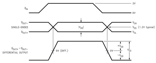
Figure 7. Driver Output Levels
