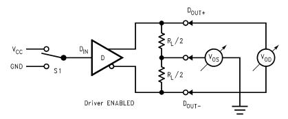
Figure 3. Driver  $V_{\text{OD}}$  and  $V_{\text{OS}}$  Test Circuit
