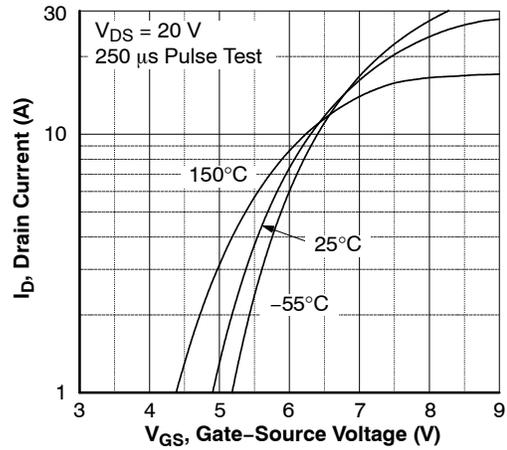
Figure 2. Transfer Characteristics
