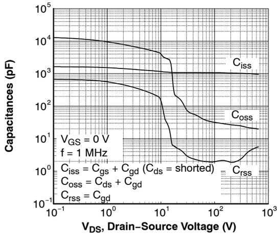
Figure 5. Capacitance Characteristics
