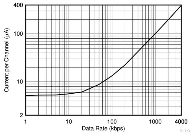
Data Rate vs Power Consumption at 3.3 V
