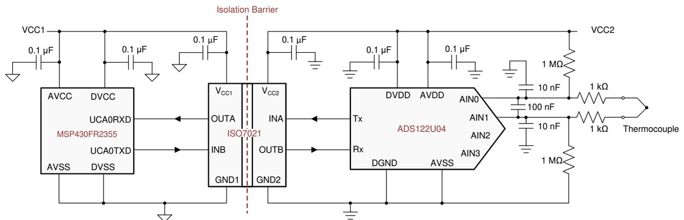
**Figure 9-3. Isolated UART for a Temperature Field Transmitter**
