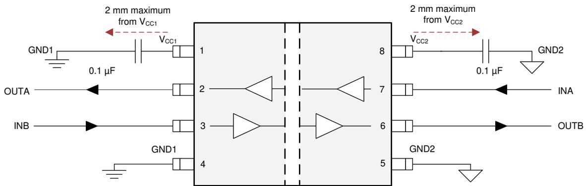
**Figure 9-4. Typical ISO7021 Circuit Hook-up**
