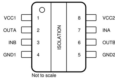
**Figure 5-1. D Package 8-Pin SOIC Top View**
