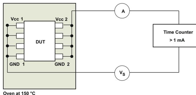
**Figure 9-1. Test Setup for Insulation Lifetime Measurement**
