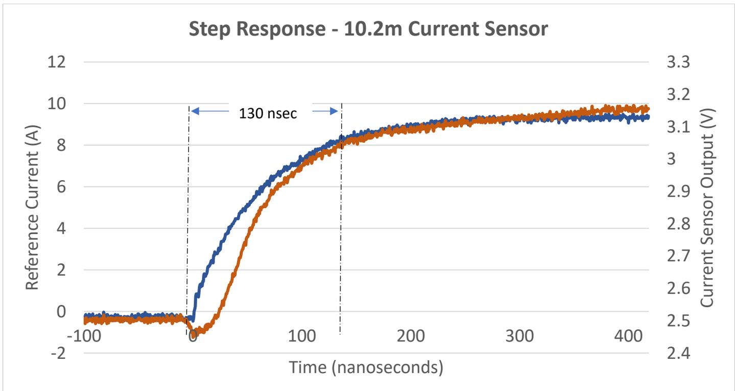
Figure 2. Step Response with 130 nanoseconds risetime.
