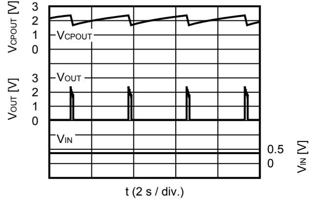
**Figure 9 Steady-state Operation Waveform for Intermittently LED Driving**
