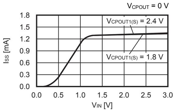
**1.5 Current consumption during operation ( $I_{SS}$ ) vs. CPOUT pin voltage ( $V_{CPOUT}$ )**
