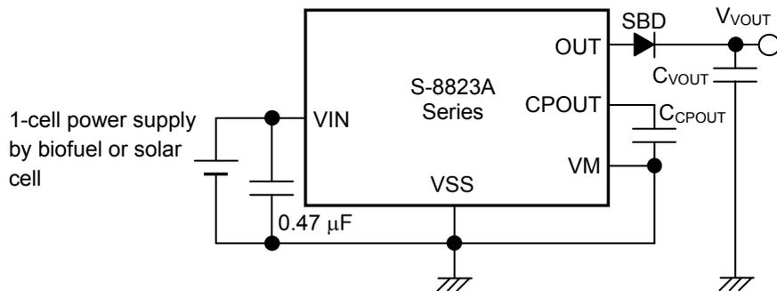
Figure 10 Circuit of Intermittently Power Supplying to Capacitor
