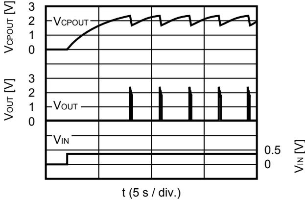
**Figure 8 Startup Waveform for Intermittently LED Driving**
