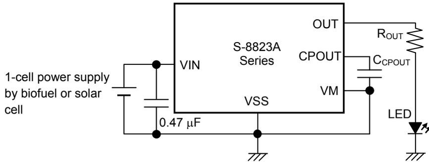
**Figure 7 Intermittently LED Driving Circuit**
