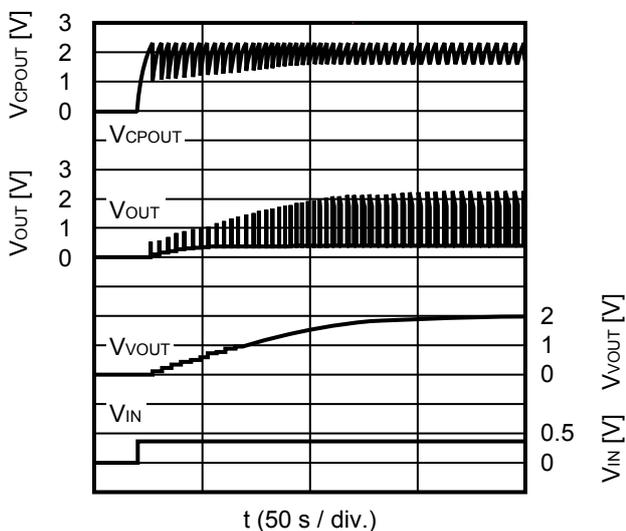
$V_{IN} = 0.37\text{ V}$ ,  $V_{CPOUT1(S)} = 2.4\text{ V}$ ,  $C_{CPOUT} = 10\ \mu\text{F}$ ,  $C_{VOUT} = 100\ \mu\text{F}$ ,  $T_a = +25^\circ\text{C}$
