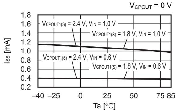
**2. 4 Current consumption during power-off ( $I_{SSS}$ ) vs. Temperature ( $T_a$ )**
