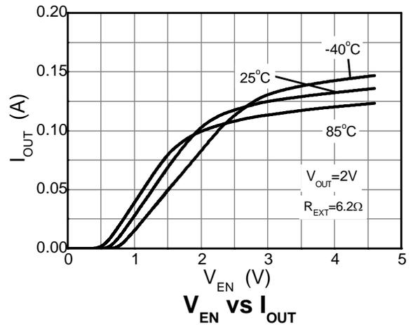
**Typical Electrical Characteristics BCR420U** (@  $T_A = +25^\circ\text{C}$ , unless otherwise specified.)
