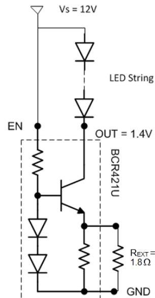
Figure 7 Example for 350mA Operation using BCR421U
