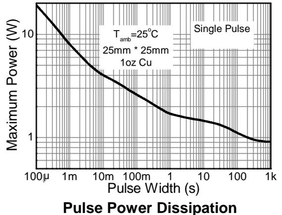
**Typical Electrical Characteristics BCR421U** (@  $T_A = +25^\circ\text{C}$ , unless otherwise specified.)
