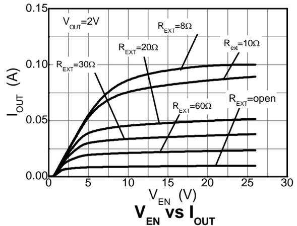
**Typical Electrical Characteristics BCR420U** (@ T<sub>A</sub> = +25°C, unless otherwise specified.) (continued)
