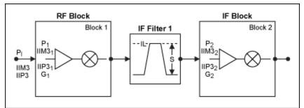
Figure 3. Block diagram for deriving the modified IP3 cascading equation. The equation incorporates the effect of adding selectivity (S) to receiver stages at the two off-channel CW tones' frequencies. Power symbols are in dBm, and gain is in dB.
