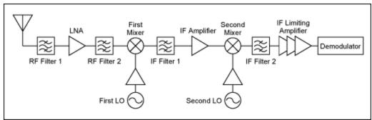
Figure 2. Conventional superheterodyne dual-conversion receiver.
