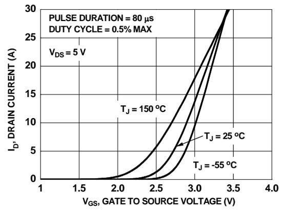
Figure 5. Transfer Characteristics
