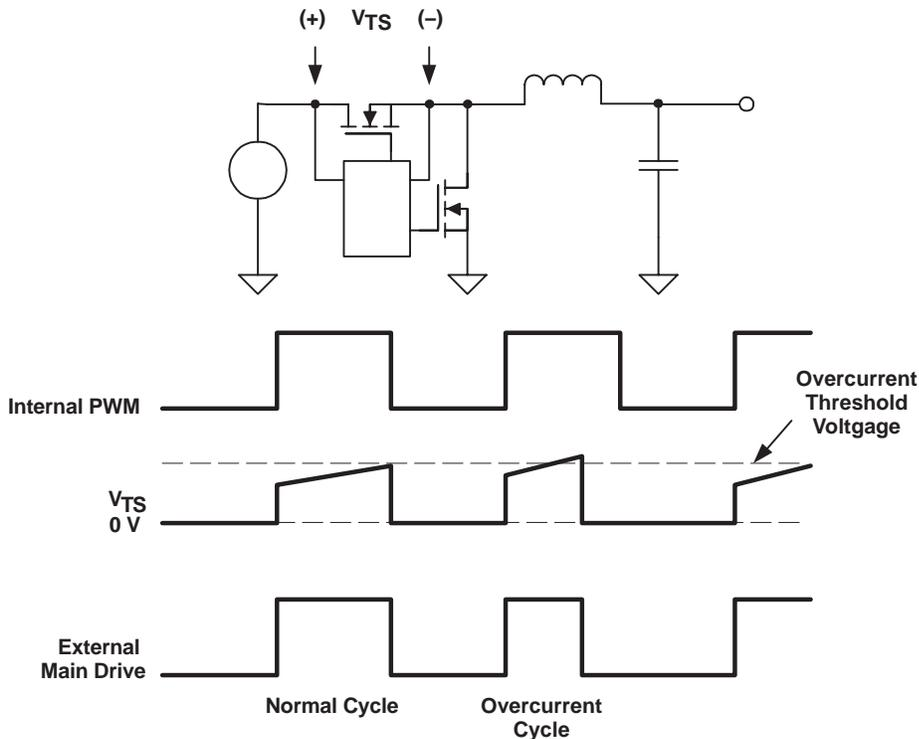
Figure 3. Switch Node Waveforms for Synchronous Buck Converter
