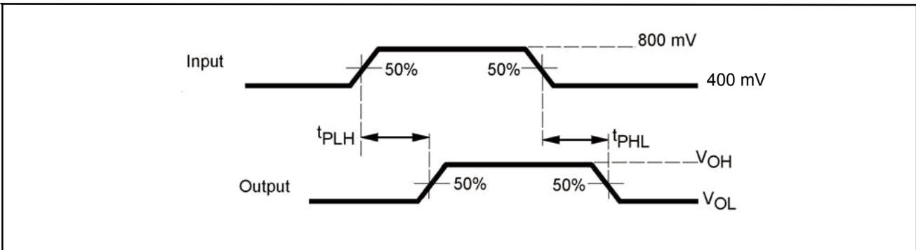
Figure 6. Propagation Delay
