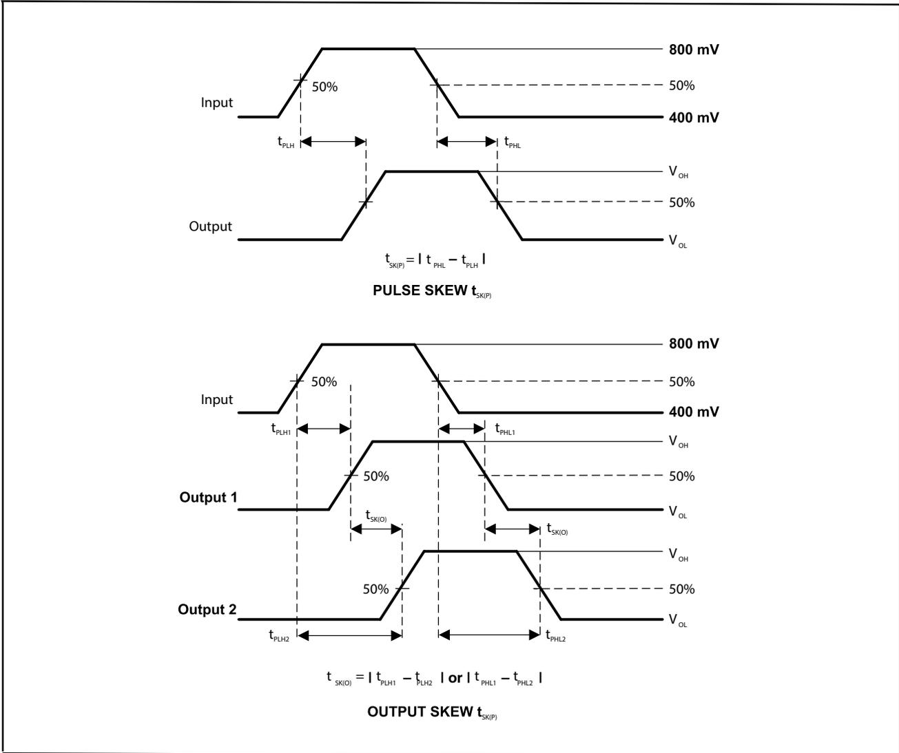
**Figure 7. Skew Test**
