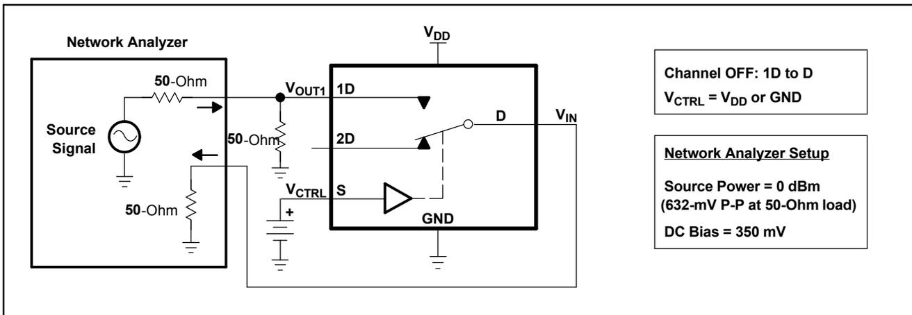
**Figure 3. OFF Isolation (O<sub>ISO</sub>)**
