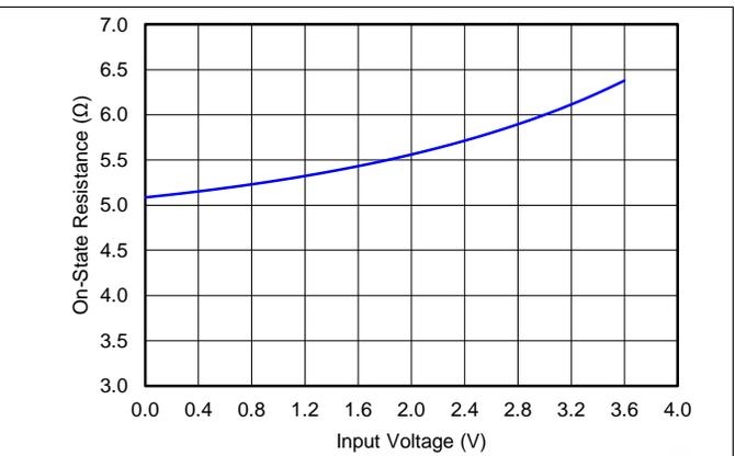
Figure 2. ON-Resistance vs V<sub>I/O</sub> for USB Switch
