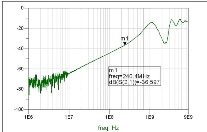
Figure 5. OFF Isolation vs Frequency for MHL Path
