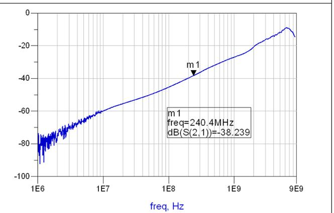
Figure 8. Cross Talk vs Frequency for USB Path
