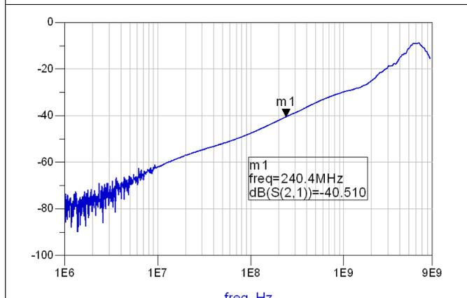
Figure 7. Cross Talk vs Frequency for MHL Path
