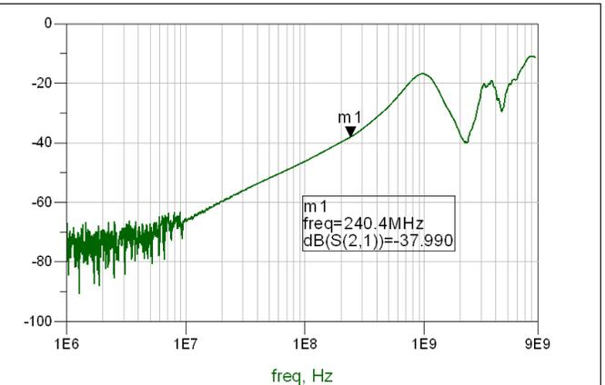
Figure 6. OFF Isolation vs Frequency for USB Path
