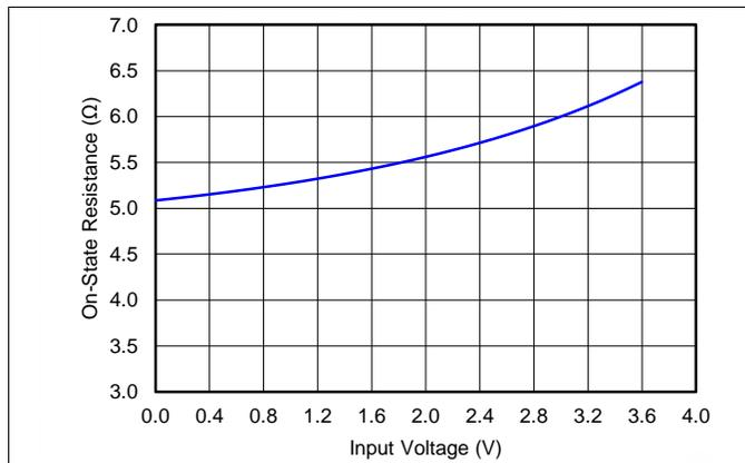
Figure 1. ON-Resistance vs V<sub>I/O</sub> for MHL Switch
