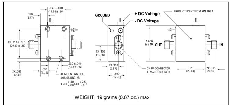
\* Dimensions are inches (millimeters)  $\pm 0.015$  (0.38) unless otherwise specified.
