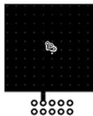
a.  $65^\circ\text{C/W}$  when mounted on a  $1\text{in}^2$  pad of 2 oz copper,  $1.5" \times 1.5" \times 0.062"$  thick PCB
