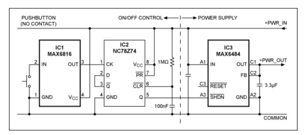
Figure 1. This normally open pushbutton connects to a debouncer, the MAX6816 (IC1) and IC2. This single-pushbutton ON/OFF control circuit lets you toggle the PWR OUT voltage by controlling the MAX6484 LDO (IC3).
