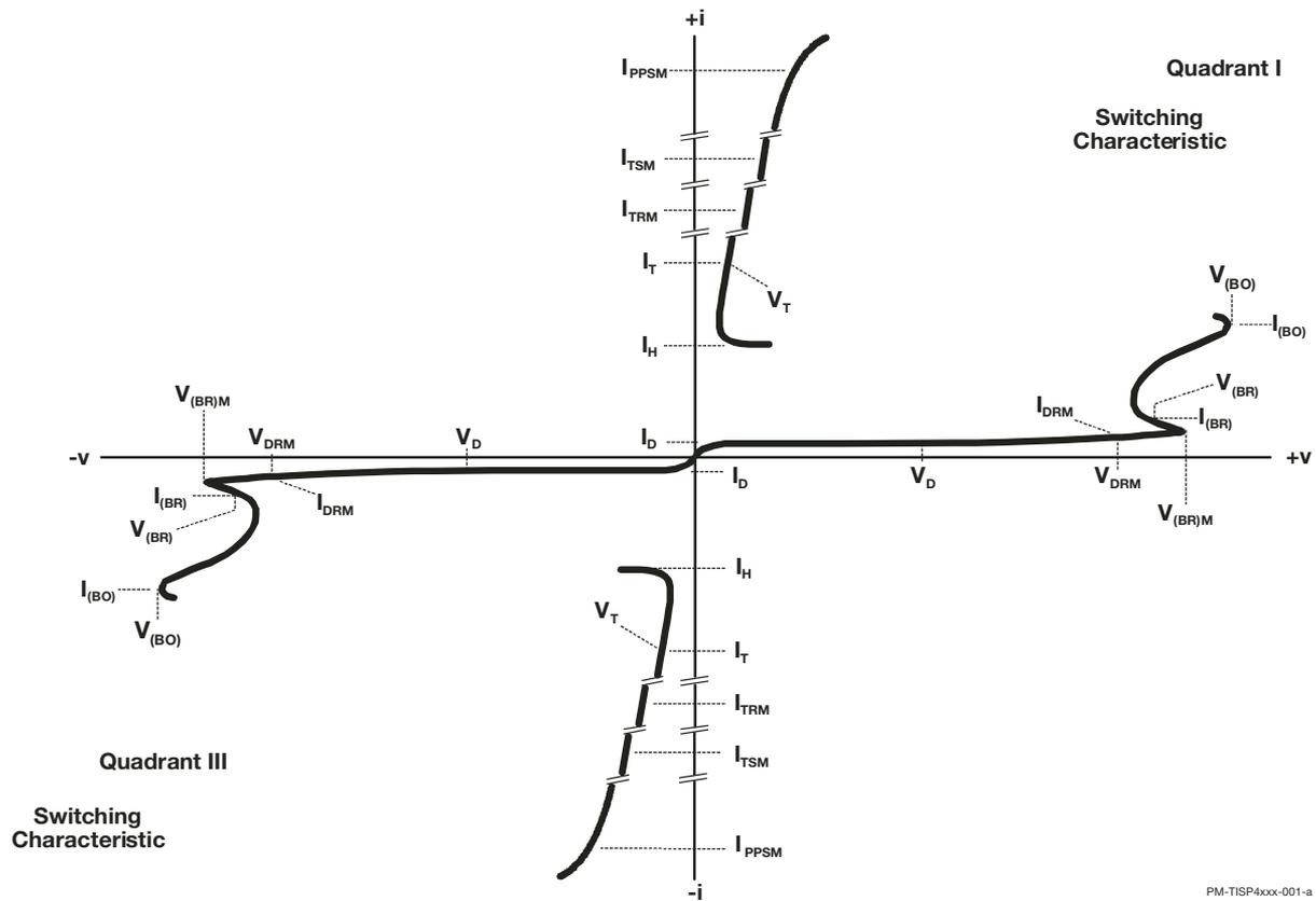
Figure 1. Voltage-Current Characteristic for the Terminals T and R
