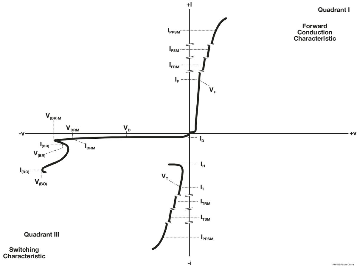
Figure 2. Voltage-Current Characteristic for Terminals T and G or R and G
