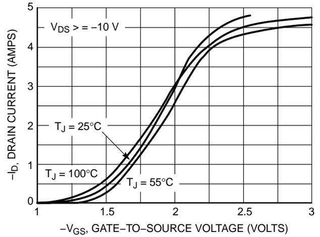
Figure 2. Transfer Characteristics.
